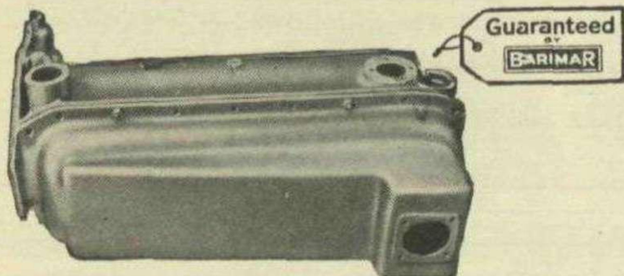
Broken parts welded in, machined and cleaned up. A perfect job which saved the customer about £25.
