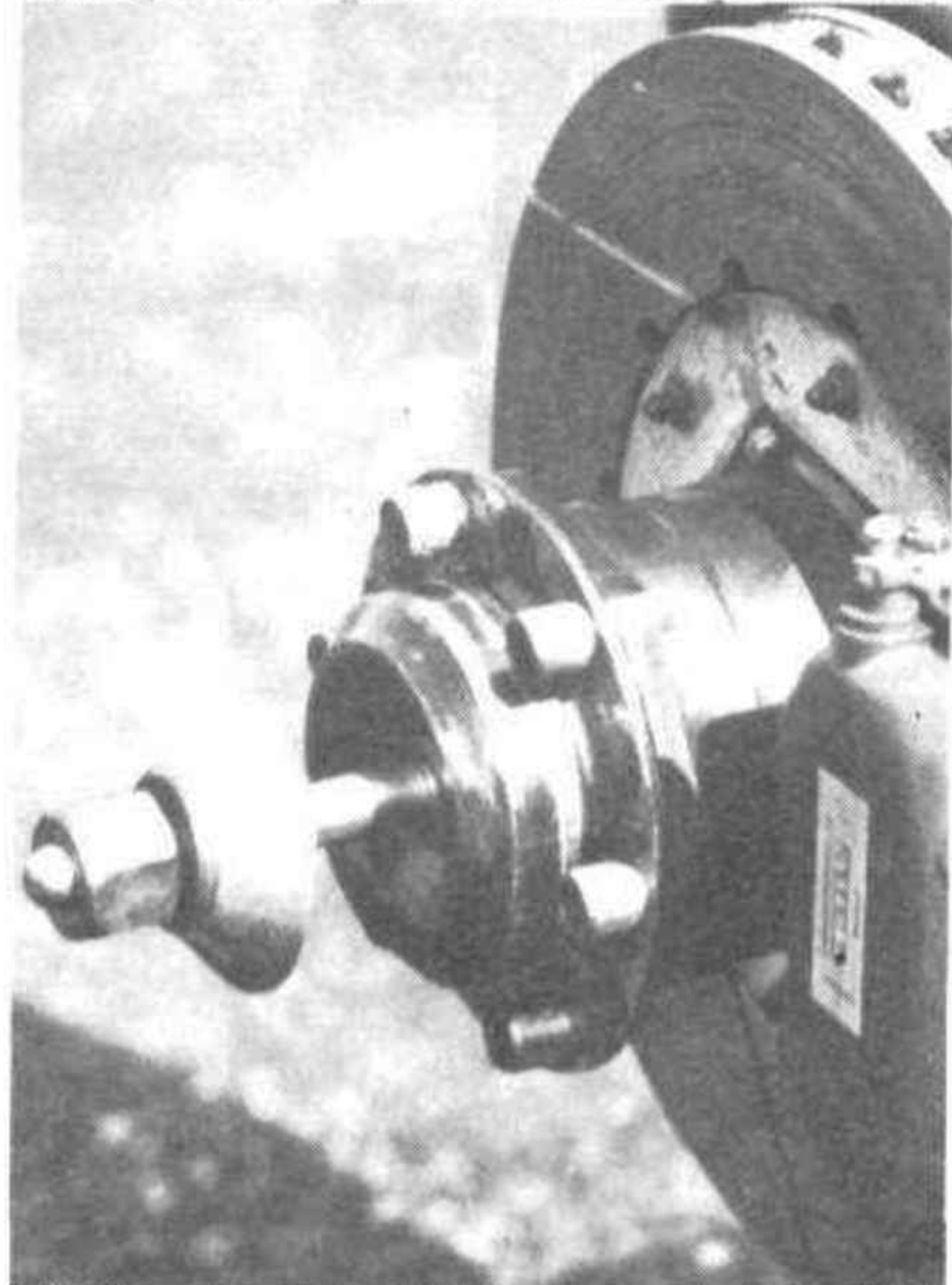
The Tyrrell uses six driving pins on the hub with a solid pin passing through the centre, the wheel being clamped to the pin flange and taper seat by the small nut and conical spacer.
