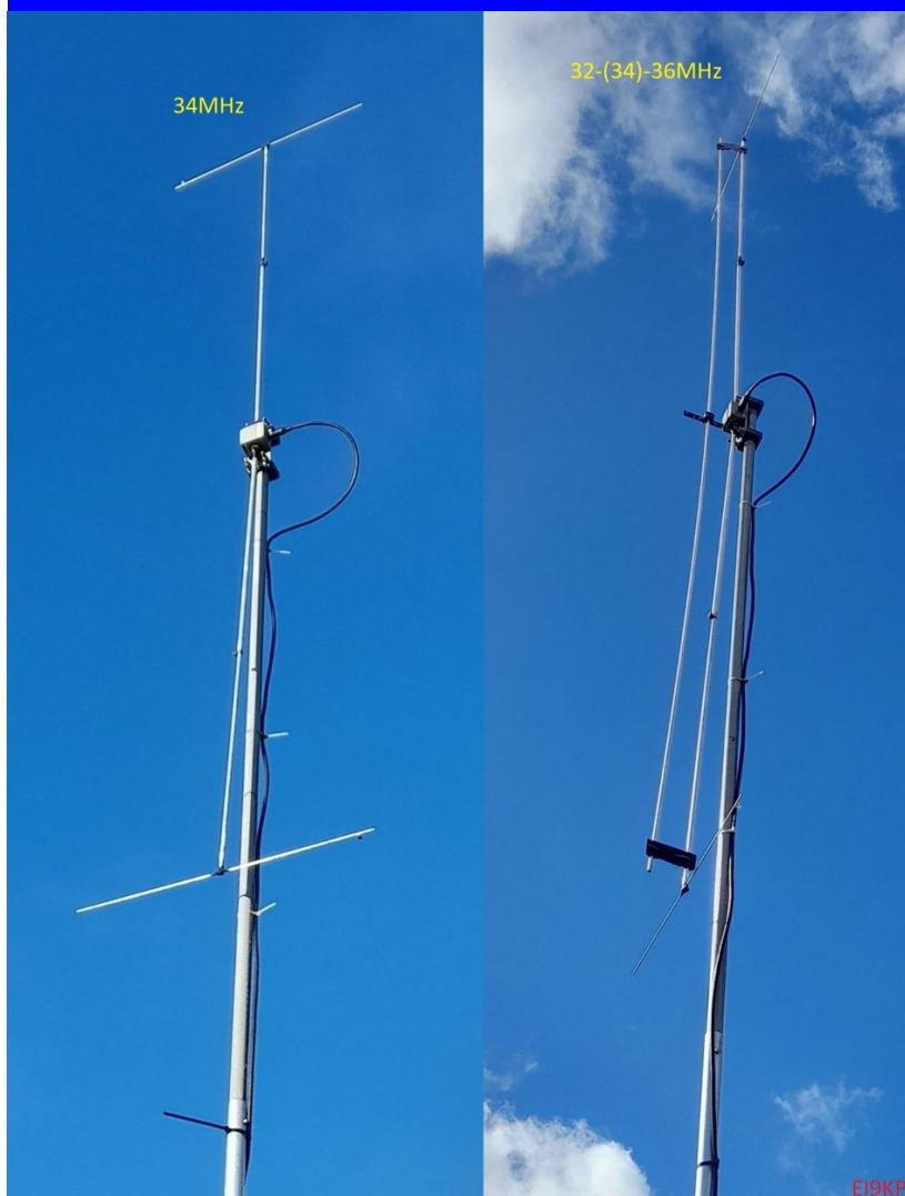
Fig. 2 L. Test Dipole with Capacitive Load R coupled dipoles for 32MHz and 36MHz
