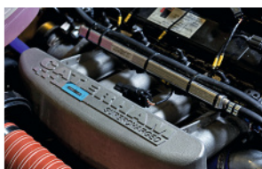
Ford Duratec motor produces 300bhp
