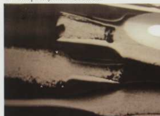
Figure 7. Magnified Xeroradiographic image of the surface find (top) and Osceola #53674 spear point (bottom). Note the many areas of porosity-bubbles and other defects attributable to casting.
