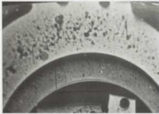
Figure 2. Xeroradiographic image of the above engine block demonstrating extensive casting porosity in the interior of the block. Note the many circular gas spaces typical of casting.
