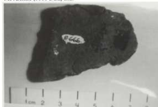
Figure 4. Riverside, MI copper artifact shown in Figure 3 and displaying a "normal" surface typical of the OCC. Internal porosity defines it as a casting.
