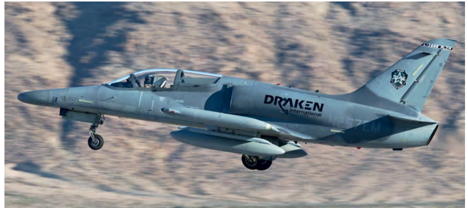
Above: Equipped with modern avionics and a potent Grifo-L pulse-Doppler multimode radar, the L-159 provides customers with a credible beyond-visual-range air-to-air threat at low cost. Joe Copalman Left: Draken's flight line at Nellis comes to life as a four-ship of A-4s prepares for an air-to-air mission in support of the Fighter Weapons School. Joe Copalman
