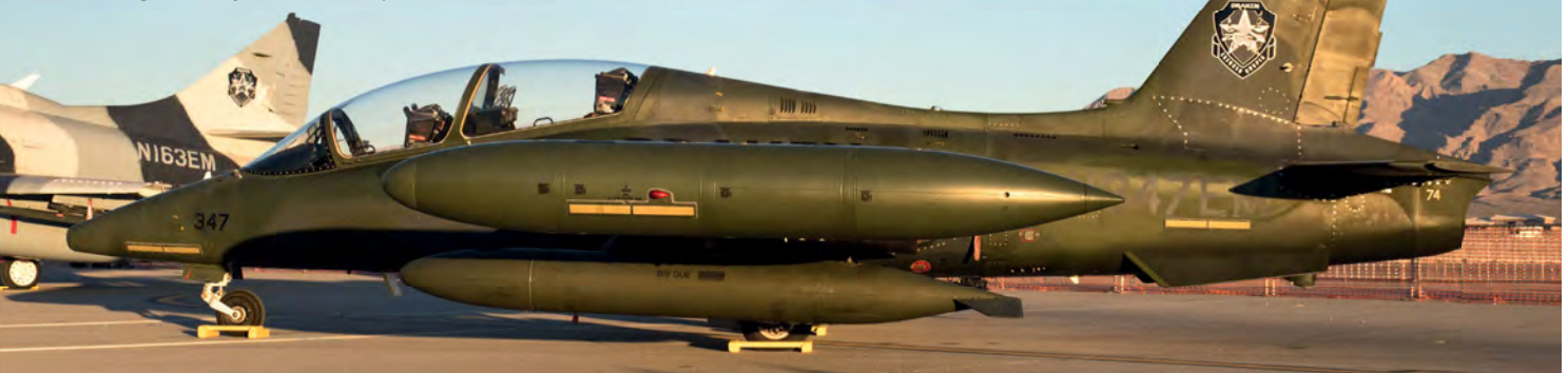
Below: Along with its A-4Ks, Draken's MB339s were purchased from New Zealand. Without radar, but having six hardpoints for air-to-ground weapons including bombs, rocket pods, and gun pods, the MB339 is an ideal, low-cost close air support training solution for JTACs. Joe Copalman
