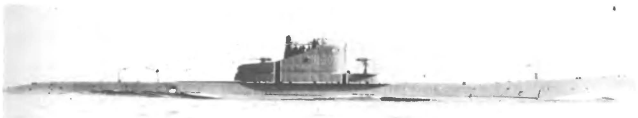
The SHCH-307 of the V- bis -2 design shown underway in the Baltic in 1939. She has 45-mm guns on a step forward of the conning tower and another on an after platform, the latter faired into the after tower casing. This unit survived World War II to have her conning tower preserved as a memorial at the submarine school in Leningrad.
