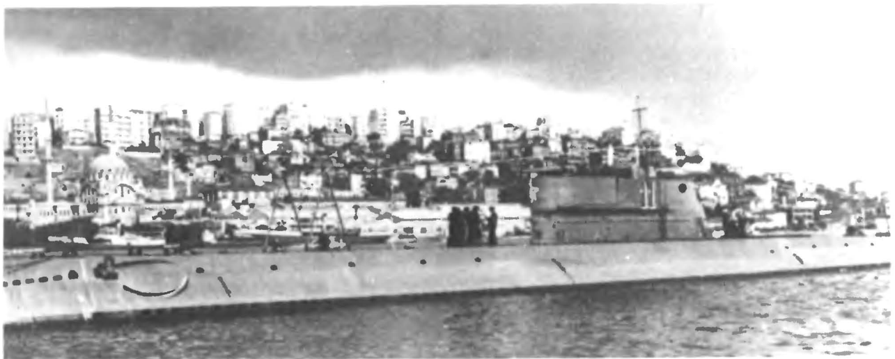
The DEKABRIST-class submarine YAKOBINETS off Istanbul in October 1933. The large submarines of the D class were built in both Leningrad and Nikolayev, this unit having been constructed in the latter's Marti (south) yard. Note the 102-mm gun mounted at the front of the conning tower, the original position of the gun. The bow planes retract into a position flush against the hull.
