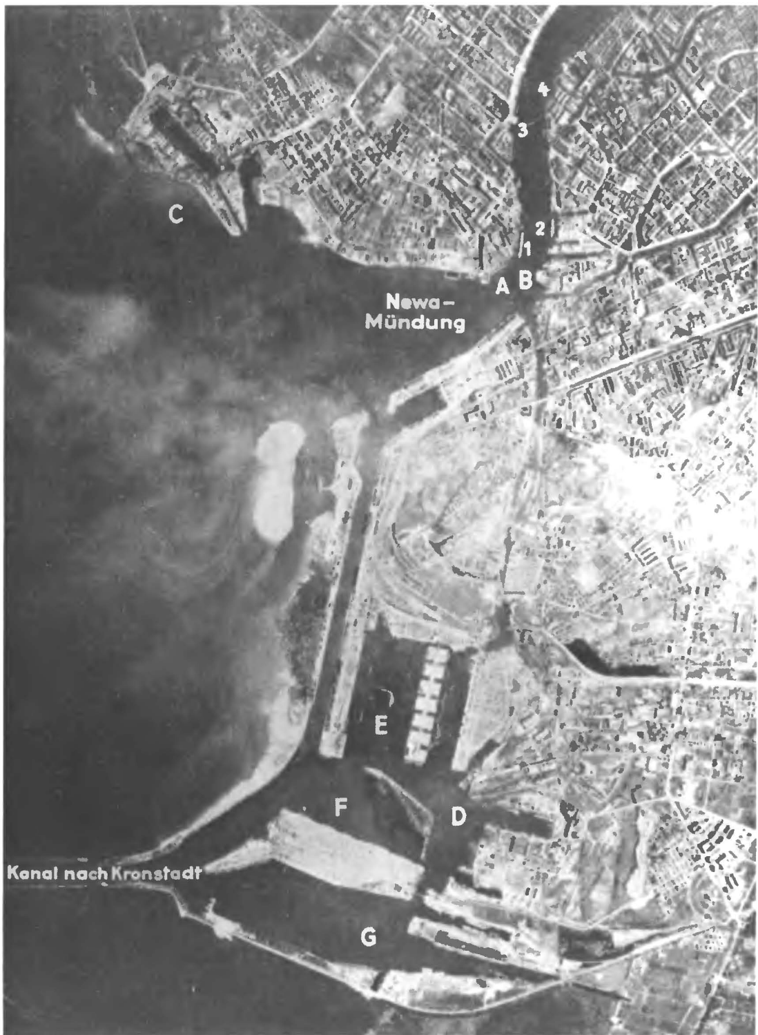
An aerial photograph of Leningrad—taken by a German aircraft in August 1941—shows the major shipyards in the city: (A) Baltic Shipyard with one battleship, one heavy cruiser, and several destroyers under construction; (B) Marti/Admiralty Shipyard; (C) wharves; (D) Zhdanov Shipyard with several destroyers being fitted out; (E) protected harbor with cargo ships; (G) coal port with one wrecked battleship and several destroyers; (1) and (2) heavy cruisers being fitted out; (3) dock; and (4) icebreaker. ( Luftwaffe photo)
