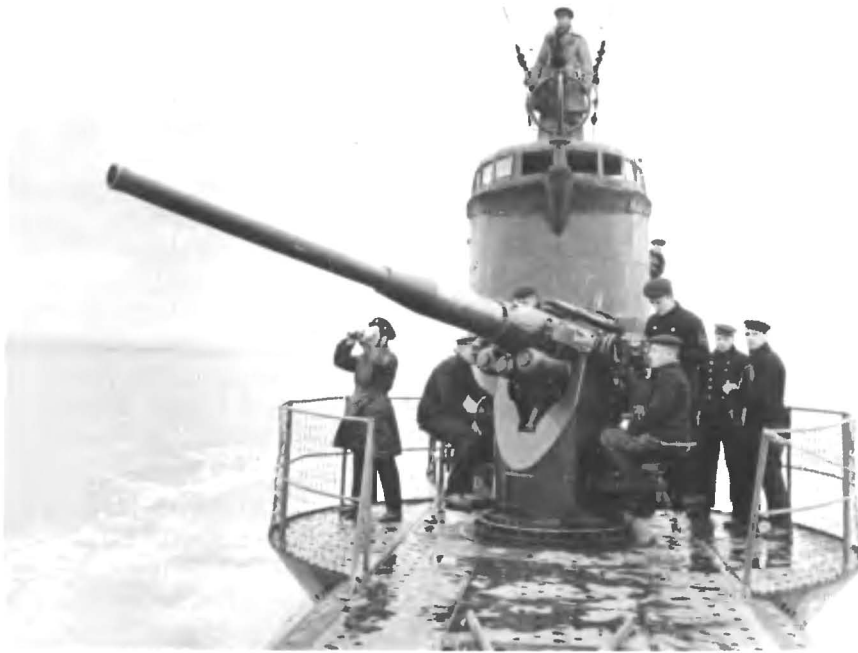
The 3.9-inch (100-mm) gun was the largest carried in Soviet submarines during World War II except for a 102-mm gun in the LENINETS class. Gunfire was the preferred—and less expensive—method of sinking small coastal craft if there was no danger of counterattack to the submarine. A radio direction finder is mounted atop the conning tower. (Sovfoto)
