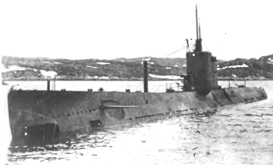
The DEKABRIST was the first Soviet submarine class, designed by a team led by B.M. Malinin. The rows of openings along the hull are limber or flood holes, indicating the craft's double-hull configuration. This is the NARODOVOLYETS in Arctic waters during World War II; her conning tower has been cut down and the gun moved down to the main deck. (Imperial War Museum)
