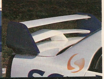
Spoiler for a fight: double aerofoil rear wing more than just cosmetic
