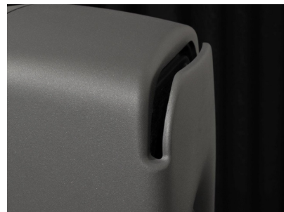
Figure 7: Acoustically concealed woofers radiate low frequency through acoustically optimized openings in the ends of the front baffle; this enables the whole front baffle to be used as a waveguide.
