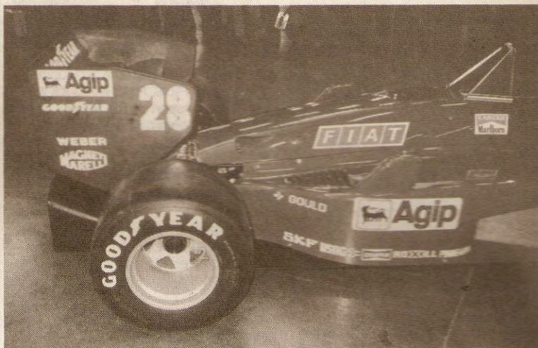
A rehoused turbo installation creates a lower, sleeker profile.
