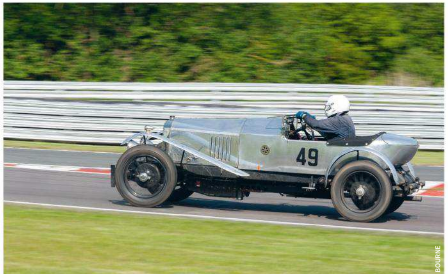
SPIRIT OF THE MEETING Assembled in 1990, Jamie Quartermaine's car might not have been the oldest on the grid, but its DNA comes from some of Vauxhall's earliest vehicles. Parts from a Vauxhall 30-98 and 23-60 form what is lovingly called 'Hannibal the Cannibal'.
