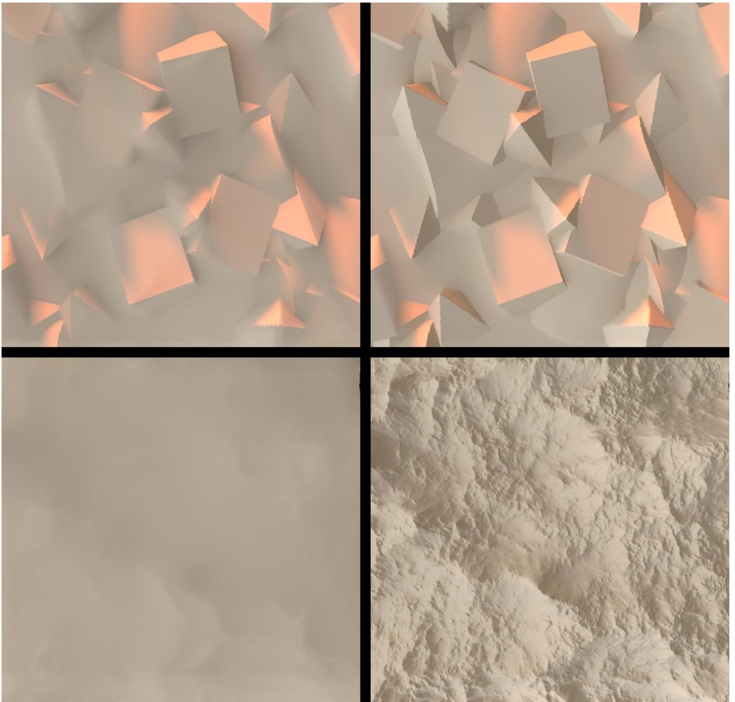
FIGURE 8. LEFT: HORIZON ANGLES ARE INITIALIZED BY DEPTH ALONE. RIGHT: HORIZON ANGLES ARE INITIALIZED WITH THE G-BUFFER'S NORMAL. WE CAN SEE THE RESULTING IMAGES ARE MUCH MORE DETAILED AND CONVINCING.
