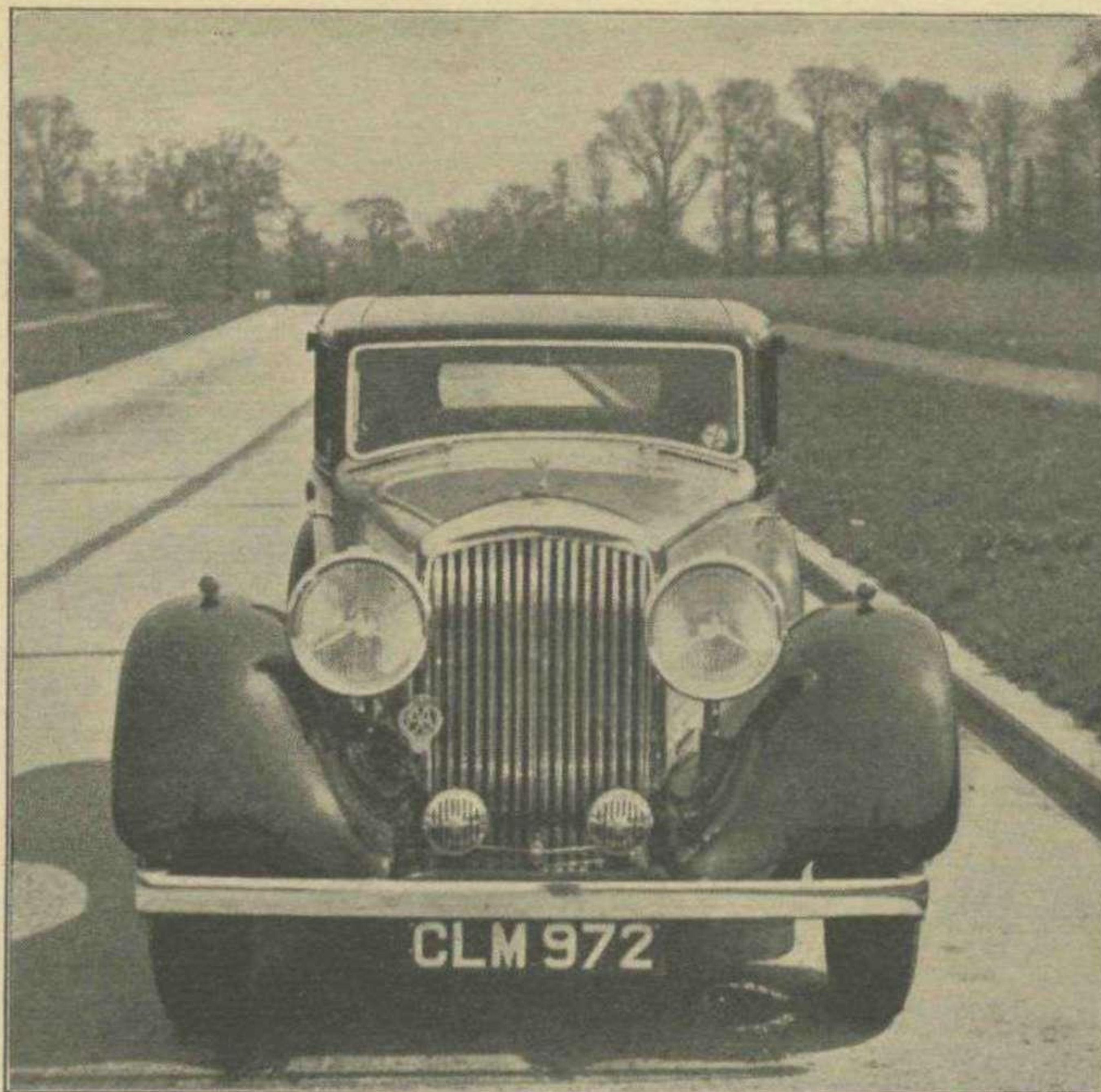
The front view of the car is enhanced by the plated radiator shutters.
