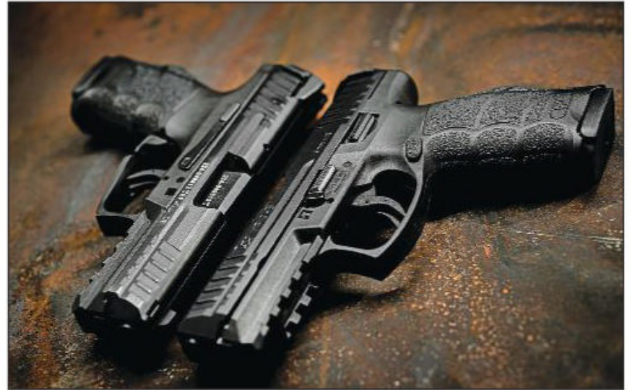
↑ Virtually identical twins, you can tell the original VP9 (left) by the paddle-style mag release, compared to the VP9-B's push-button release.
