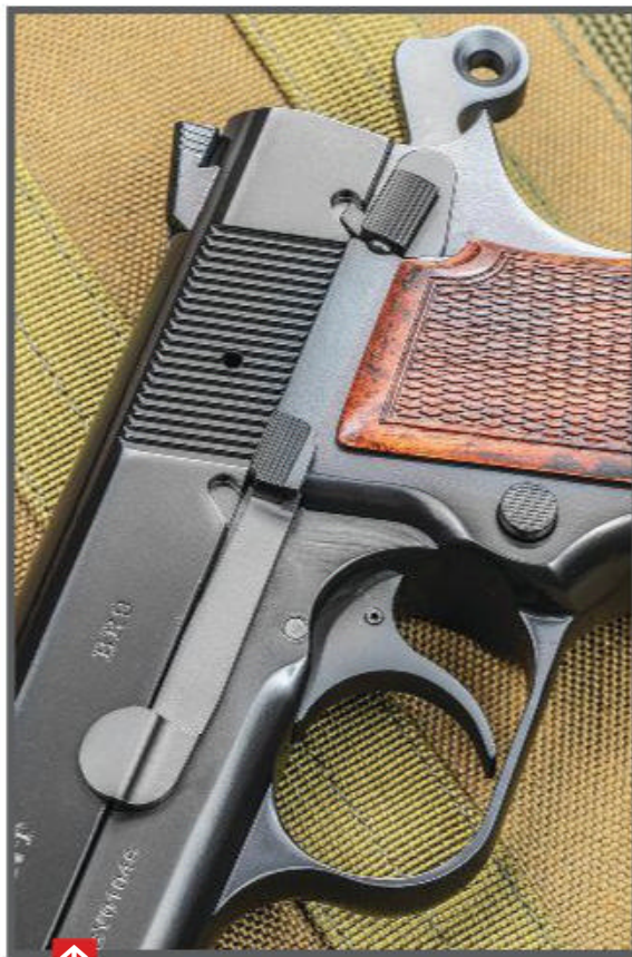
While the author initially thought the glossy black finish was blued steel, it is actually a rugged Cerakote finish.
