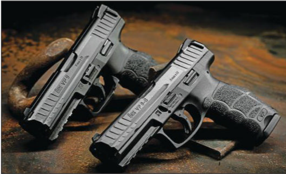
↑ Virtually identical twins, you can tell the original VP9 (left) by the paddle-style mag release, compared to the VP9-B's push-button release.
