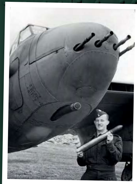
LEFT An armorer holds up a 6Pdr shell under the nose of the so-armed Tsetse Mosquito. (MARY EVANS PICTURE LIBRARY)
