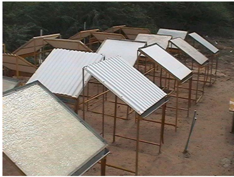
Figure 20. Different types of condenser surfaces investigated by [55].
