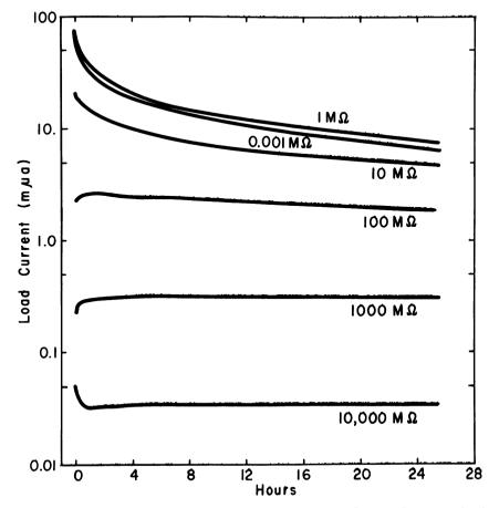
Graph 1. Current levels obtained from silver-platinum couplings with various levels of interposed resistors. Measurements were made *in vitro* with a Hewlett-Packard 425A microvolt ammeter with electrodes immersed in normal mammalian saline. Not only is the steady state current altered by the resistor, but the initial current drop is markedly changed as well.
