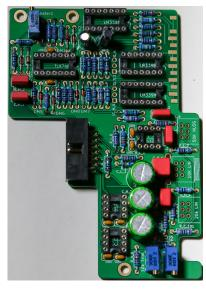
At this point we should clean our board and give the board and us a bigger break. Cleaning boards can be done with alcohol/water/your preferred method. But don't clean the Board after Trimpots, Switches and Pots are installed. Trimpots, Switches, Potentiometers don't like cleaning and that can lead to problems with electrical contact.
