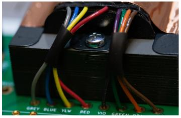
Place the Input Transformer with a gap between PCB and transformer. You can use a space or just solder one pin and later the other pins.
