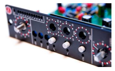
Check the alignment of the Switches and the Pots from upside again and try to align it to the silkscreen as good as possible. After that install the bracket on the Mainboard to make sure everything is in place.
