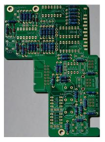
After Placing and Soldering all Resistors, we solder the next bigger parts like IC-Sockets and small capacitors, like Yellow 100nF and capacitors next to IC Sockets.
