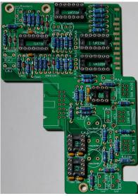
After that Step solder all Wima Capacitors, Electrolytics and Board Connectors as on the pictures.
