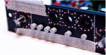
Now it's time to use the Frontpanel for the first time to get the Switches and LEDs in place. Use the spacers and bring the Frontpanel in place with just the Mainboard. You should use the nuts to screw them together. Install the pushbuttons and rearrange the switches on the PCB until they are in the middle of the hole of the Frontpanel. After this process you can solder them in completly. After soldering in all of the Pots and Switches make sure that their leads are also trimmed short.
