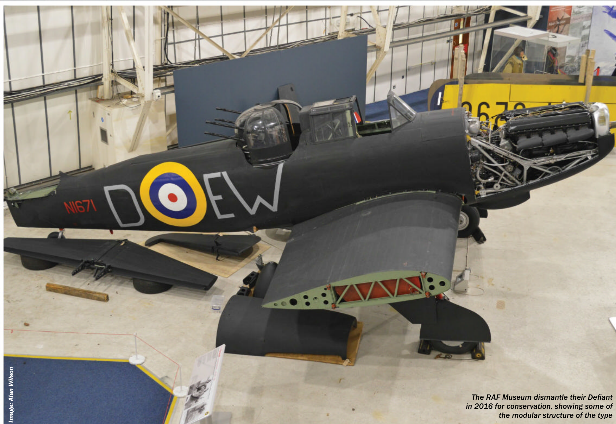
The turret area of the Defiant needed extra structural support, and a mechanism to retract the faring (as here) to allow complete movement of the guns
