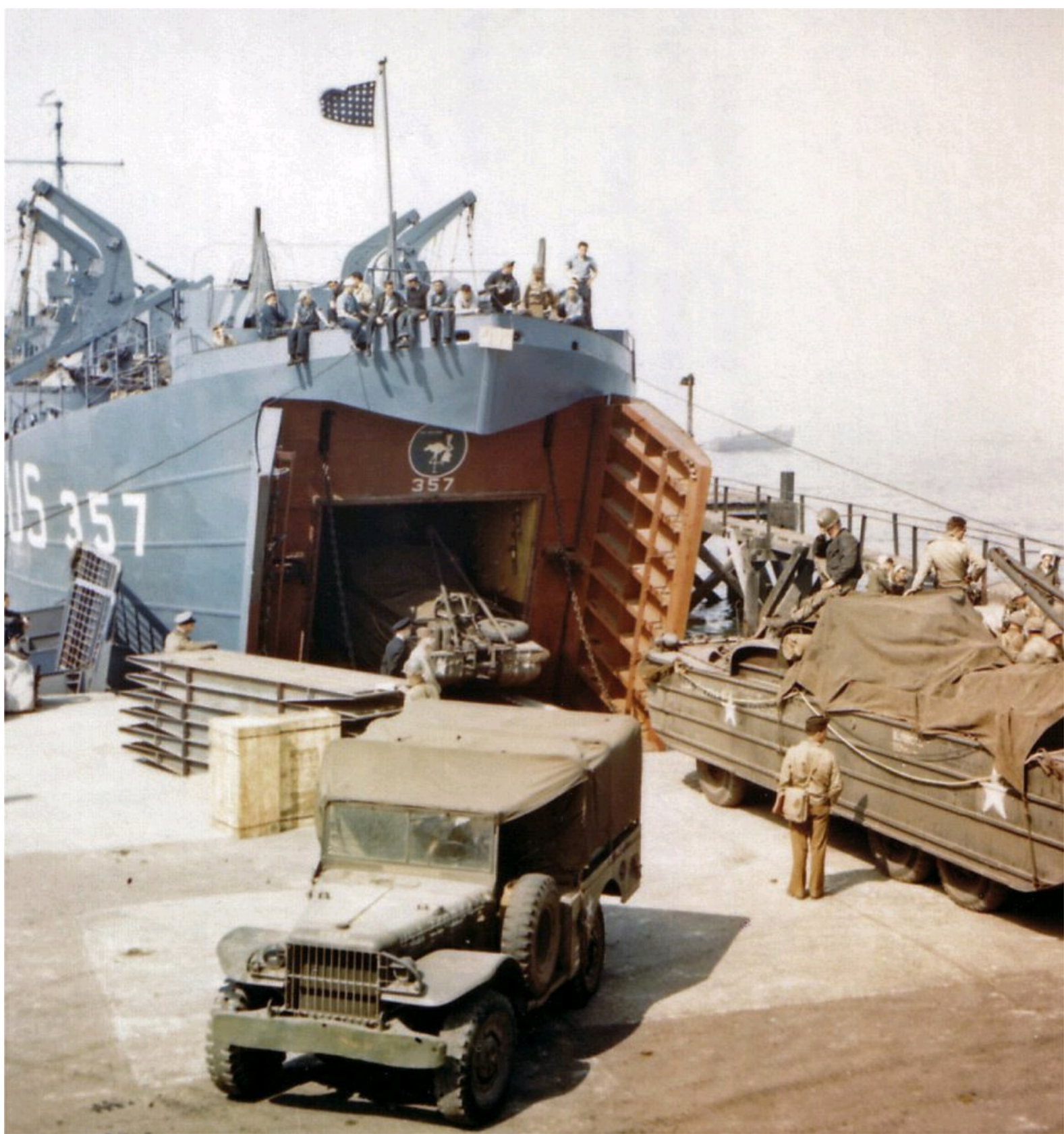
Loading LST-357 at Portland Harbour in Dorset during embarkation before D-Day. In the foreground, a Dodge WC-51 Winchless Weapons Carrier and a GMC DUKW 353 2.5-ton amphibian truck prepare to come aboard. The emblem above the throat leading to the ship's tank deck depicts a stork (nicknamed "Palermo Pete") and the motto "We Deliver." By June 1944, LST-357 had already participated in the Operation Husky landings in Sicily (July 1943) and the Operation Avalanche landings at Salerno, Italy (September 1943). On D-Day, "Palermo Pete" landed elements of the U.S. Army V Corps on the Easy Red sector of Omaha Beach.
