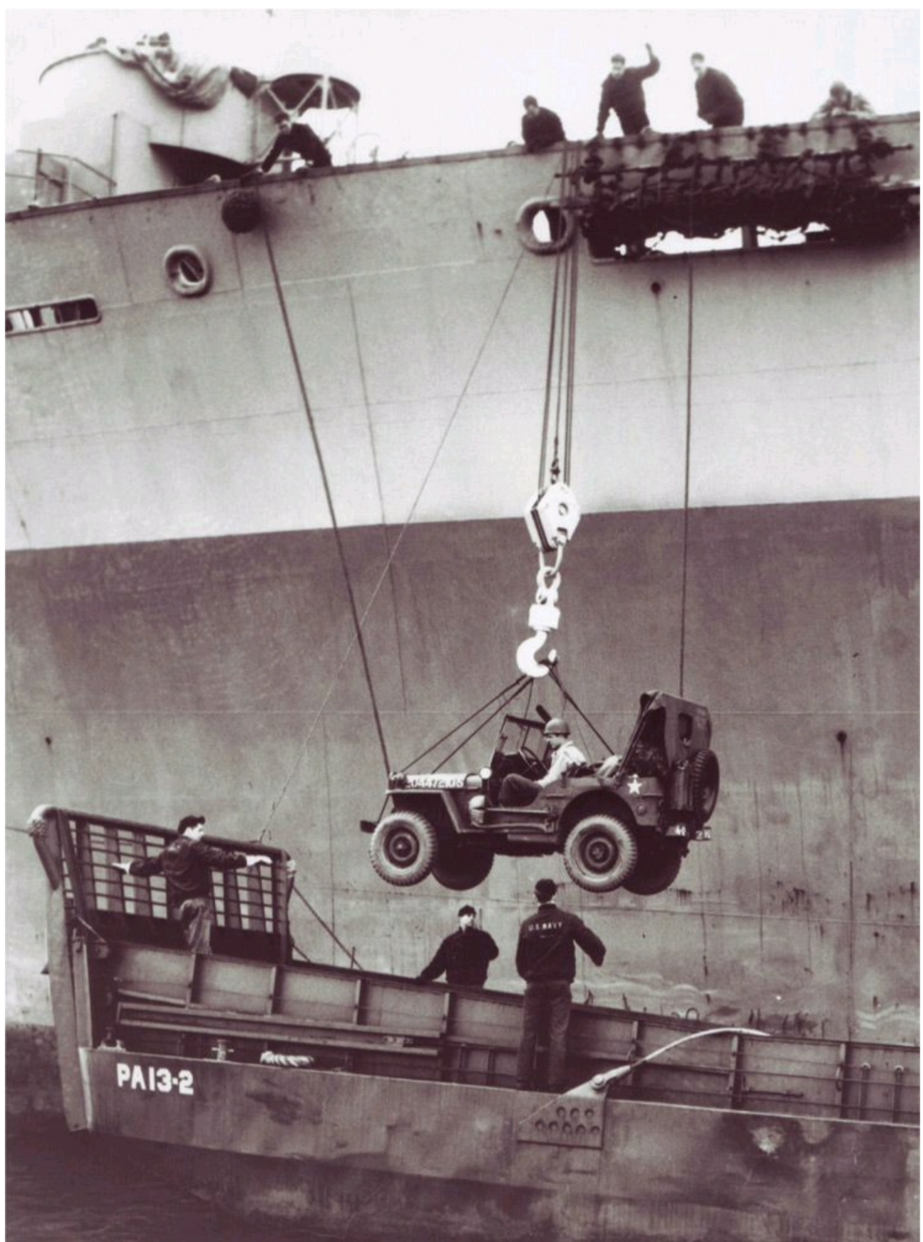
A Jeep is lowered onto a Higgins Landing Craft, Mechanized (LCM)-3 from the Harris -class attack transport USS Joseph T. Dickman (APA-13).
