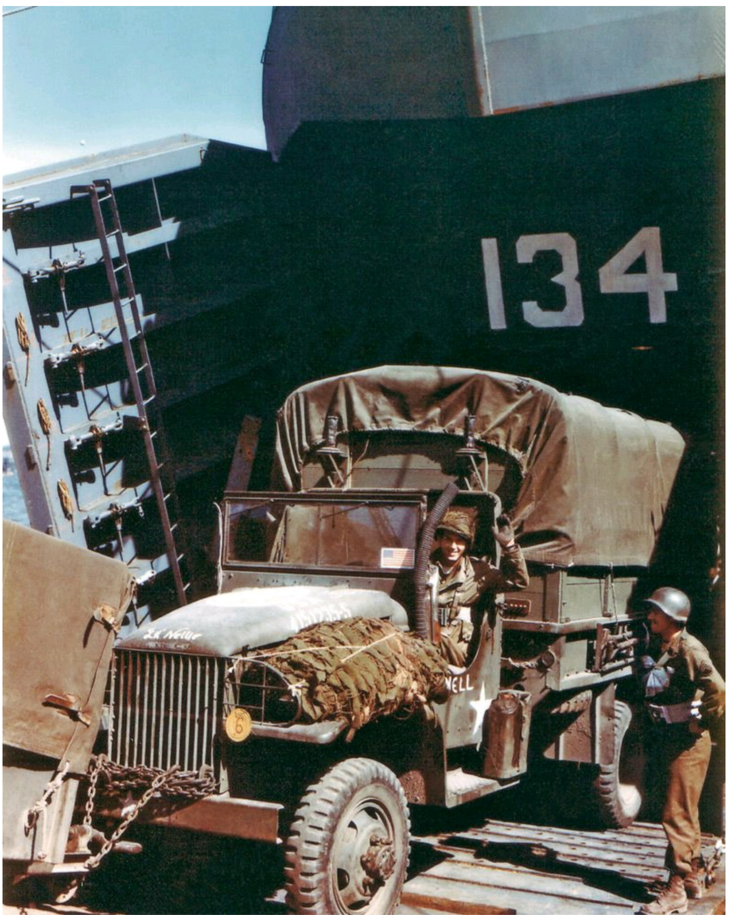
A GMC CCKW 353 2.5-ton truck nicknamed "Lil' Nellie" is loaded aboard LST-134 at Portland Harbour in Dorset during embarkation before D-Day. A deep-water fording kit has been installed on "Lil' Nellie," and she has a camouflage net lashed to her left front wheelwell. LST-134 carried elements of the divisional headquarters for the 1st Infantry Division to the Easy Red sector of Omaha Beach on June 6, 1944.
