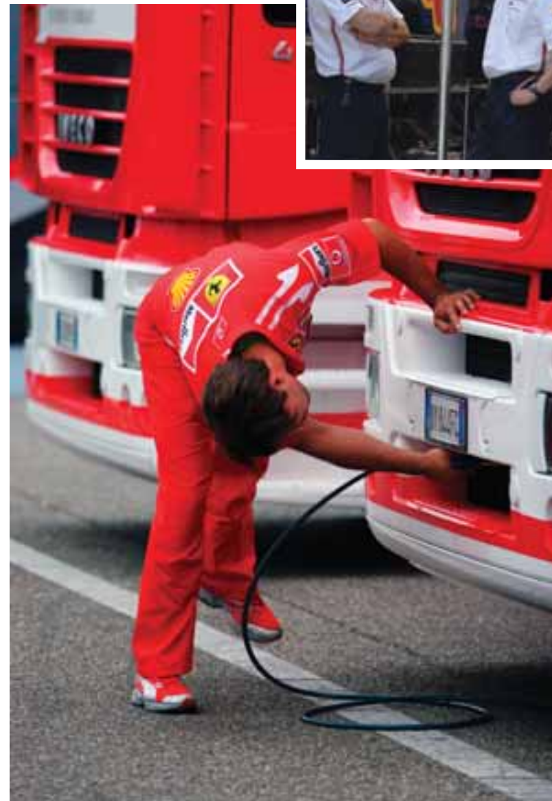
HIGH-TECH FERRARI level their trucks using compressed air.....
