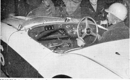
TROUBLE for Protheroe: (Above) His offside front stub axle broke after the second hour, but he drove back to the pits on three wheels and drove over the line to finish. Note the brake disc in the cockpit.
