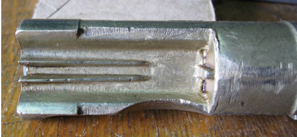
Original cast bronze STEN bolt:
