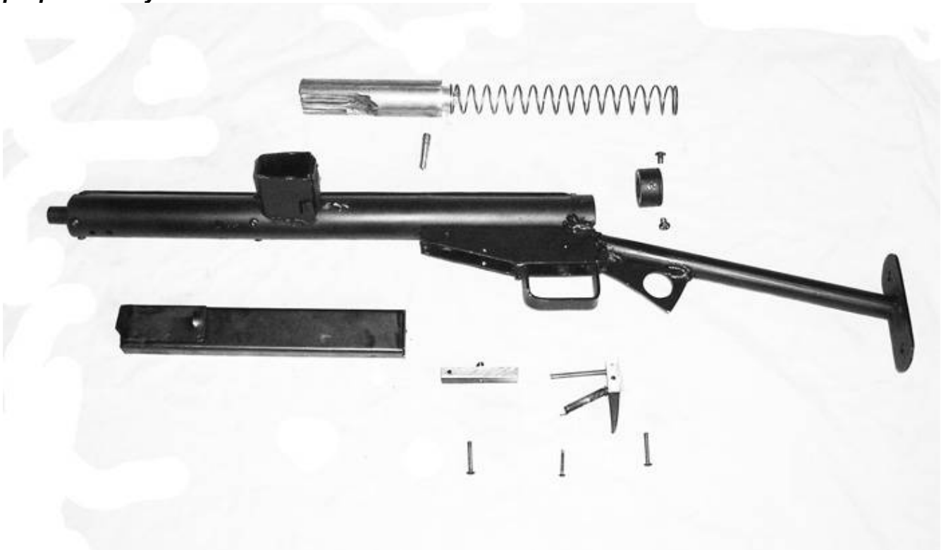
(Disassembled: Back plug, recoil spring, bolt, magazine, sear and trigger displayed)
