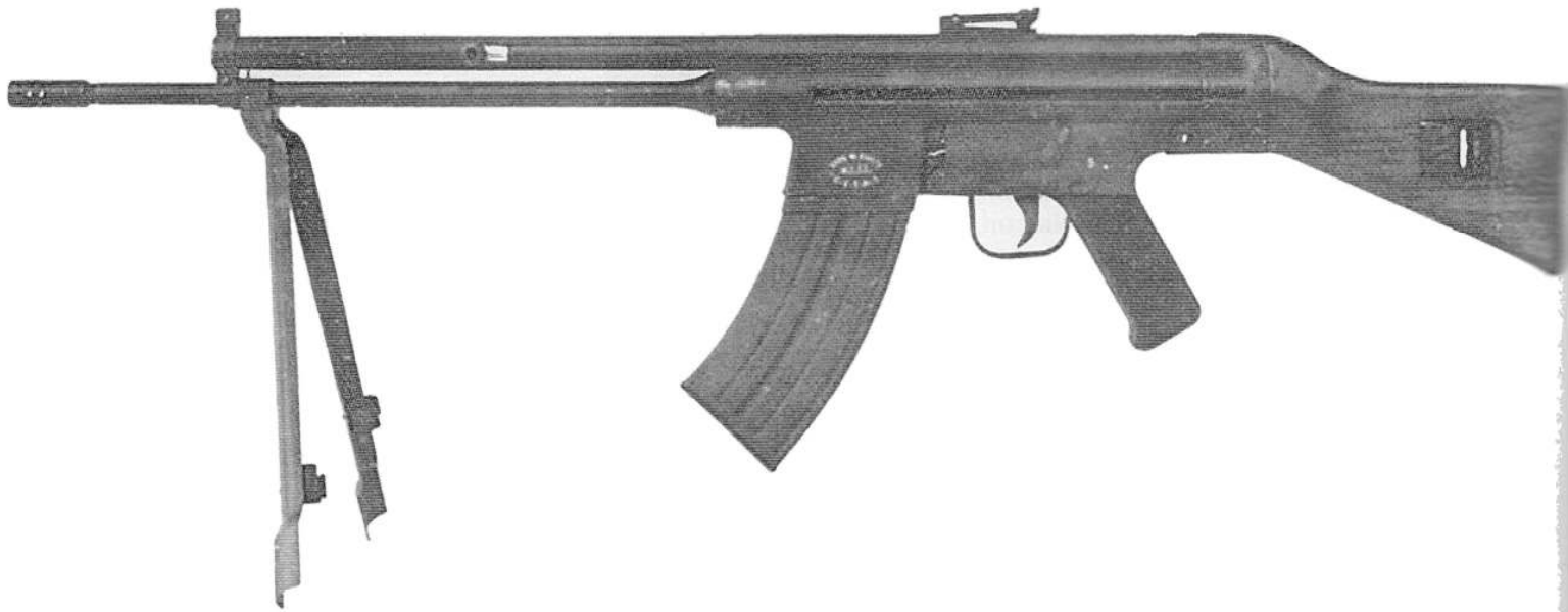
149. Left side view of the roller-locked CETME Modelo 2 , designed by Ludwig Vorgrimler, who due to obstacles put in his way by the French did not arrive in Madrid until nine months after the CETME programme had begun. In
