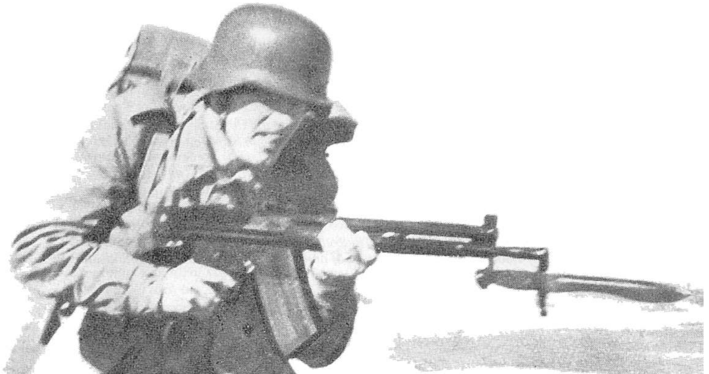
155. Another illustration from the May, 1954 CETME handbook, intended to show off the proposed versatility of the CETME assault rifle. Here a prototype is fitted with a Spanish Mauser "bolo" bayonet, mounted under the barrel muzzle. courtesy Nigel Hinton
