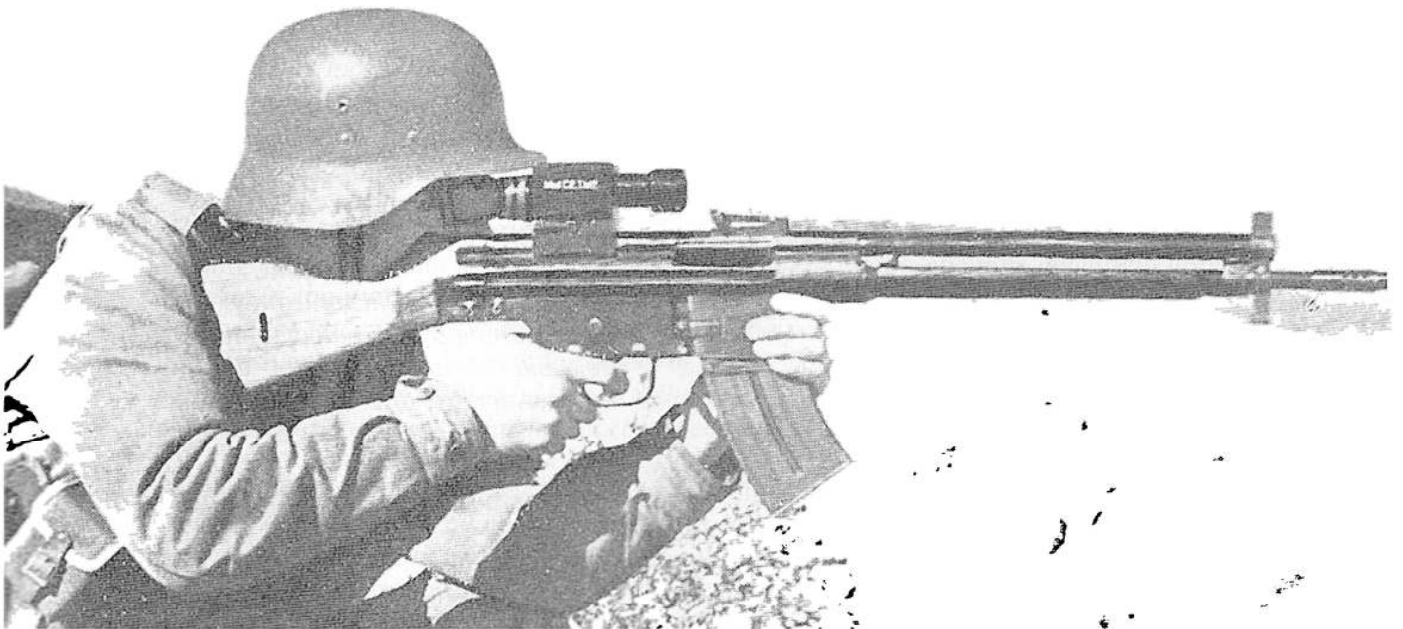
156. A final illustration from the May, 1954 CETME handbook, showing the prototype fitted with a mockup of an optical sight. Note the bayonet lug under the front sight block, and the rebated front end of the flash hider, dimensioned to accept the ring on the bayonet crossguard. Neither of these features appear on later versions. courtesy Nigel Hinton
