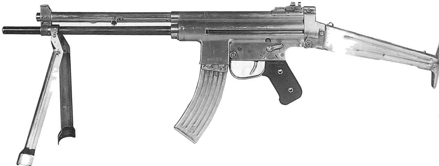
131. Left side view of the Löffler Model II/2 prototype, in calibre 7.62x33mm fitted with a design-specific 40-round magazine marked "Mod. II/2".
