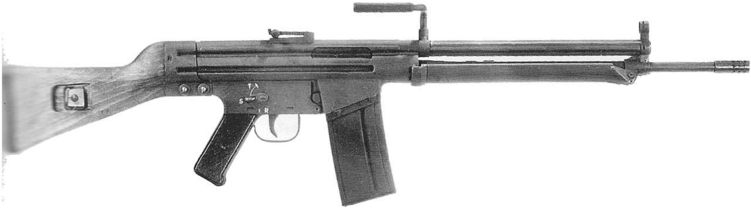
Right side view of a CETME Model A, shown with bipod folded and carrying handle raised, fitted with 15-round magazine.
