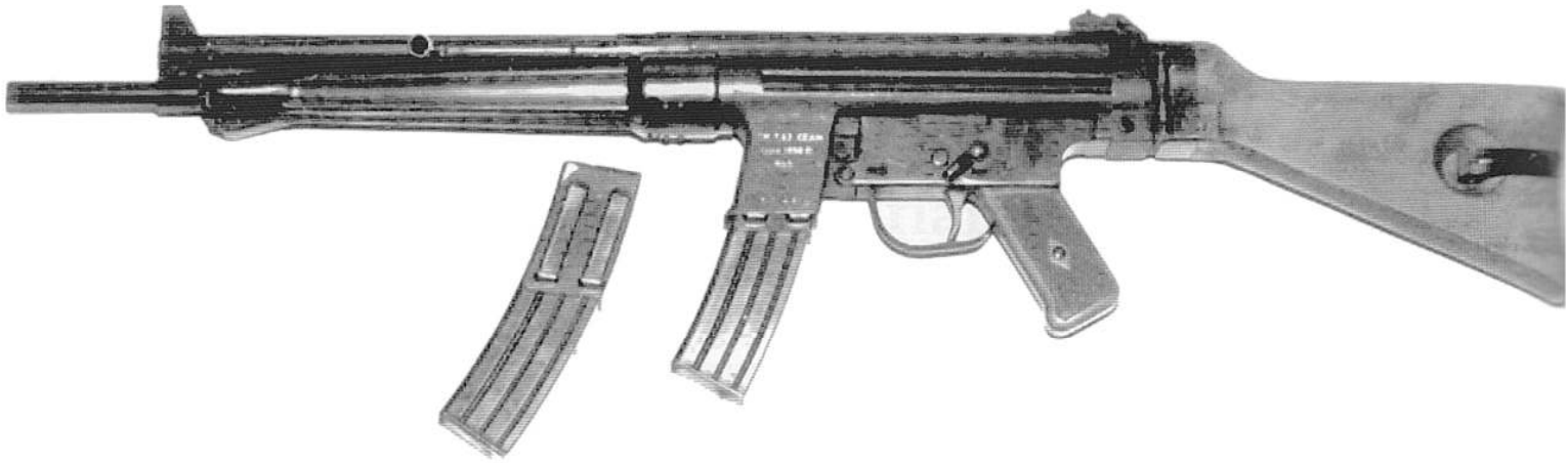
142. Left side view of Model 50 carbine serial no 5, with bipod folded and a spare 30-round magazine included.
