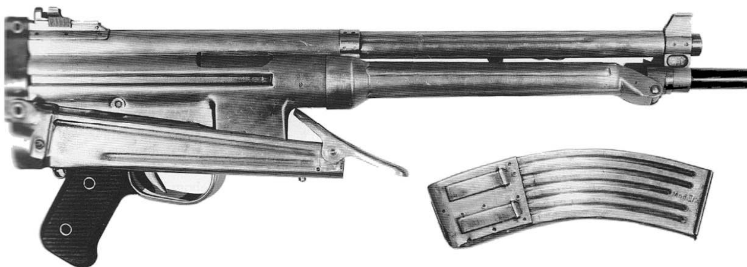
132. Right side view of the Löffler Model II/2 prototype, with butt and bipod folded.
