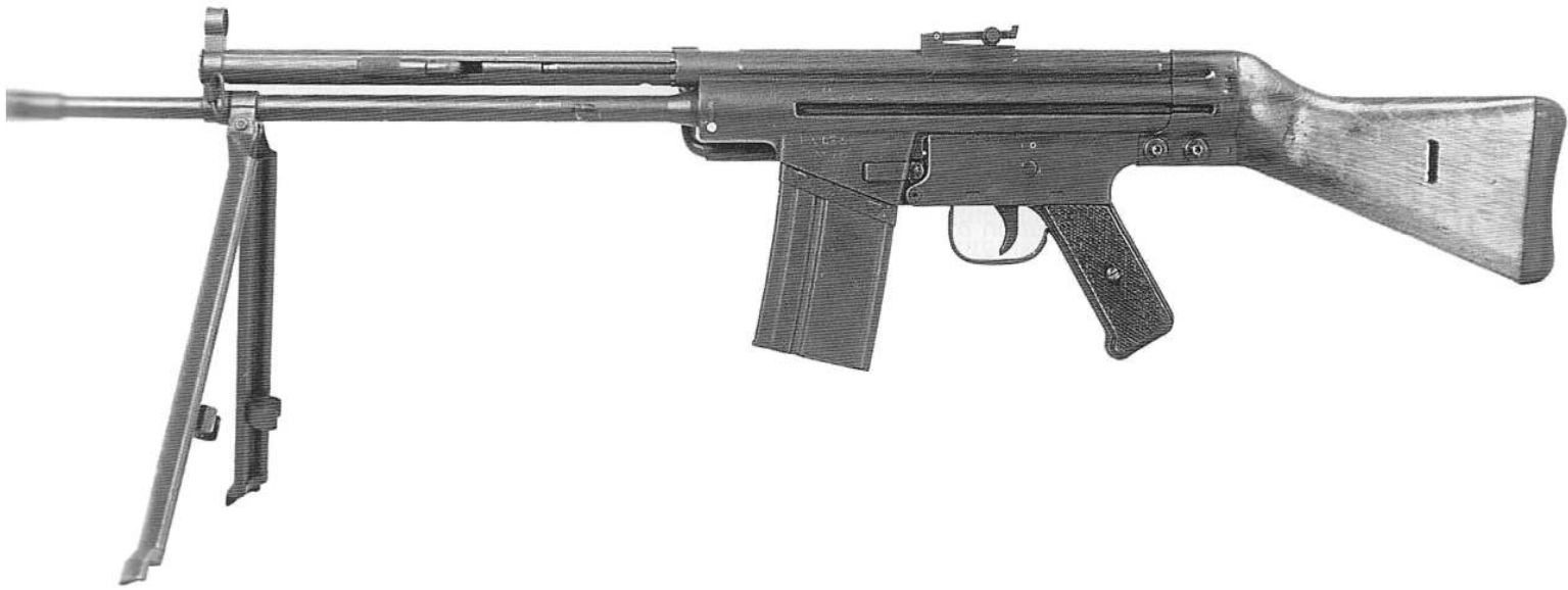
Fig. 154. Left side view of the CETME Model A, marked on the magazine well "FA CETME/A-585", shown with bipod lowered.
