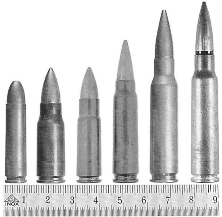
After reworking these projectiles at Satory by reshaping the bullet to the correct ogive and resizing to restore correct diameter, the trials continued.
