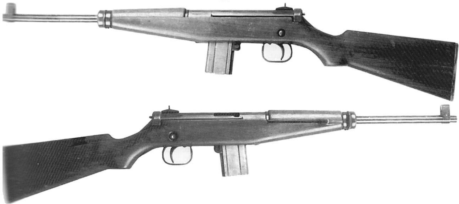
129. Left and right side views of the Vorgrimler self-loading carbine, a roller-locked arm constructed in calibre 7.62x33mm (.30 US carbine) in accordance with Project
