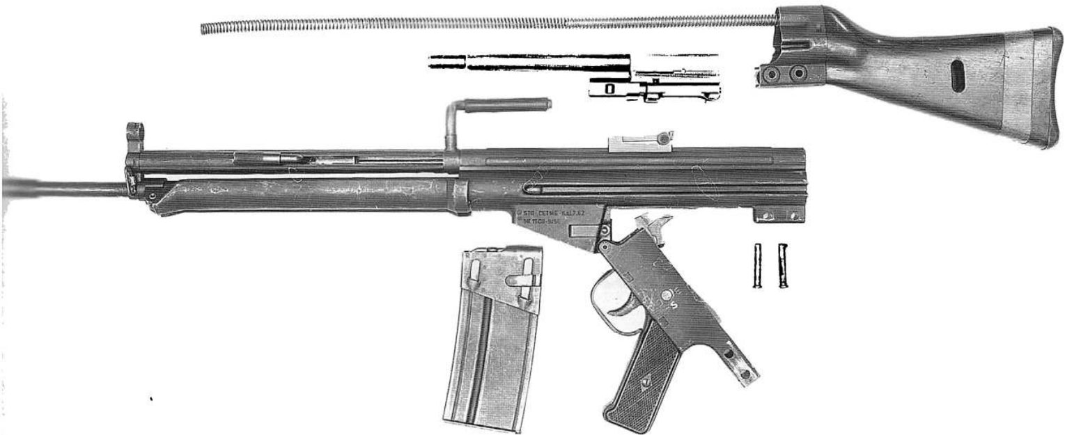
217. Left side view of STG CETME serial no 1508, produced in September, 1956, with butt pins removed, butt assembly, bolt group and 25-round magazine disassembled, and trigger group lowered.
