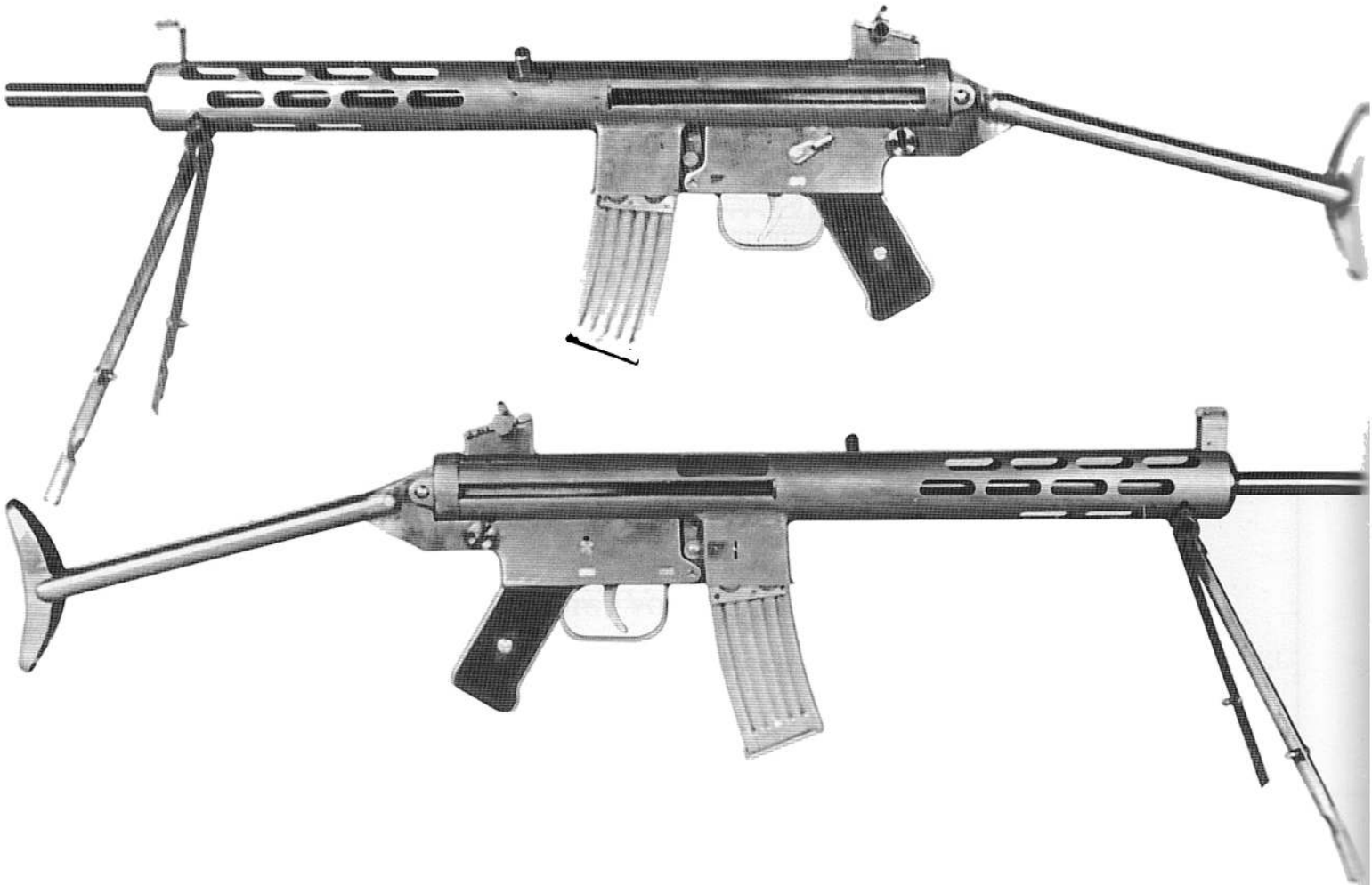
116. Left and right side views of Ludwig Vorgrimler's Model I carbine, chambered for the Model 1948 7.5x35mm French short cartridge, showing butt and bipod extended.
