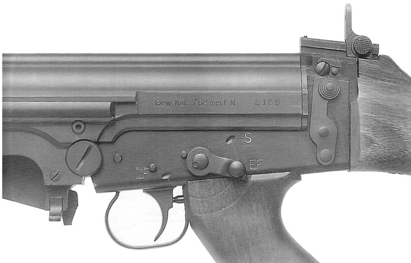
181. Left side closeup of FAL “Canada” serial no 2168, typical of the first of two deliveries to the Bundesgrenzschutz , fitted with wood furniture, high sights, and hand-tuned triggers.
