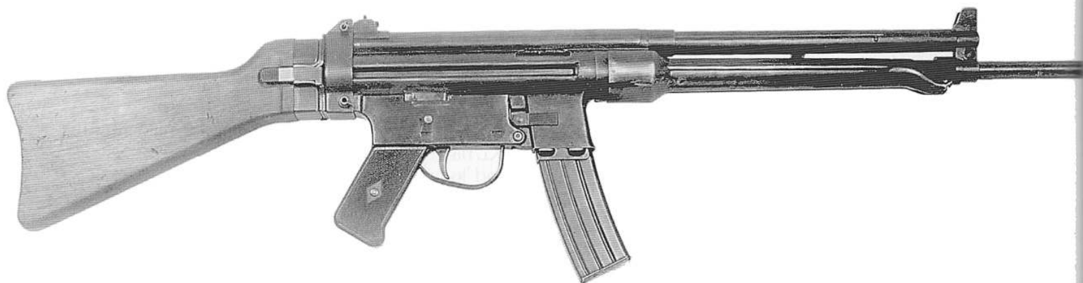
134. Right side view of the transitional Löffler Model II/3 which became the first Model 1950 carbine in January, 1950, shown with butt open and bipod folded.
