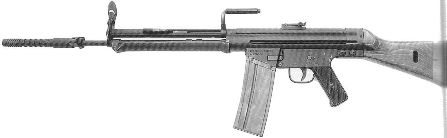
219. Left side view of STG CETME serial no 1512, also produced in September, 1956, with grenade launcher and grenade sight installed.
