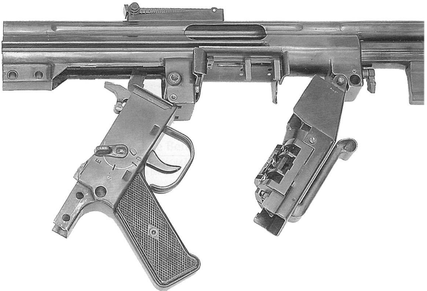
226. Right side closeup of Mauser-CETME machine gun serial no V-011 with grip and feed assemblies lowered.
