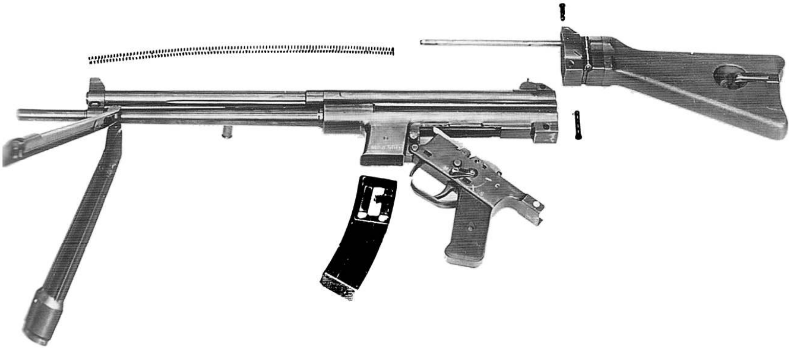
140. Left side view of the Model 50/1, partially stripped. The butt pin has been removed, the butt, captive recoil
