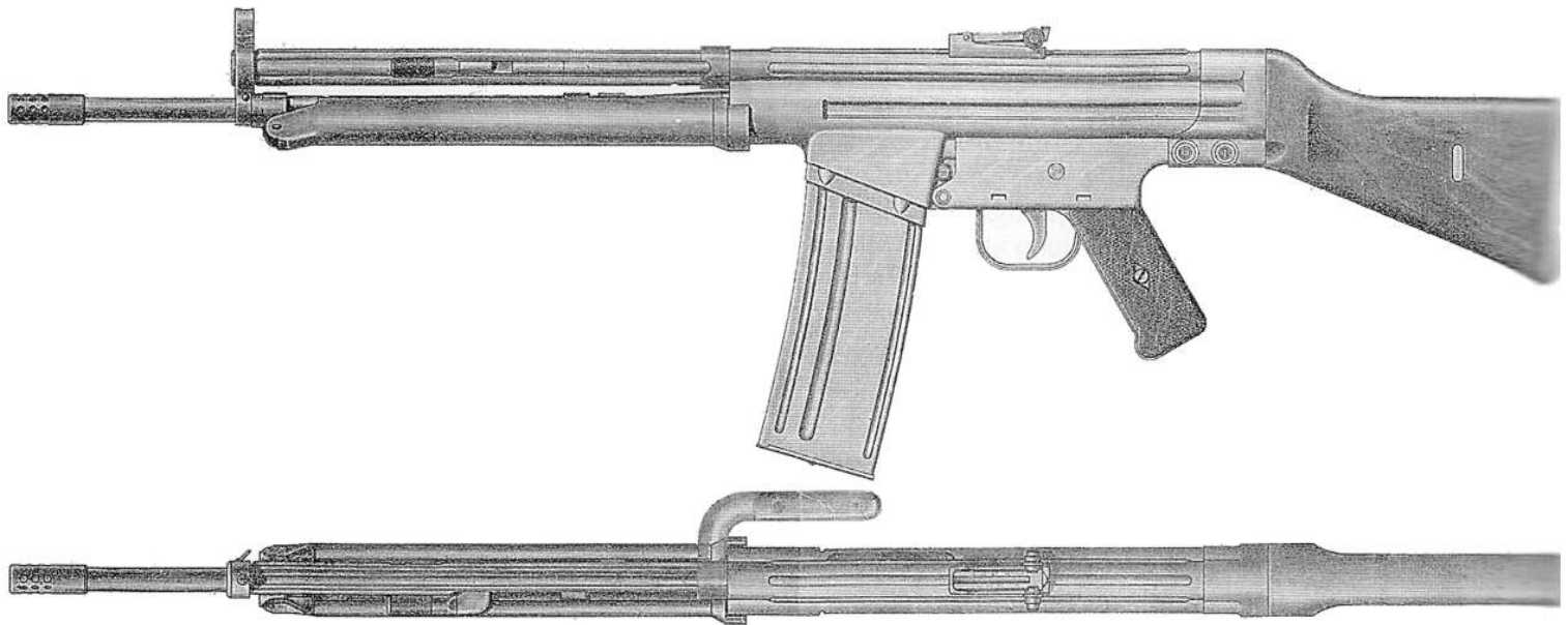
188. A reduction of a CETME wall chart titled Fusil de Asalto (Assault Rifle) depicting the Model A CETME, 400 of which were ordered in April, 1956 to be produced by H&K in Germany for Bundeswehr trials.
