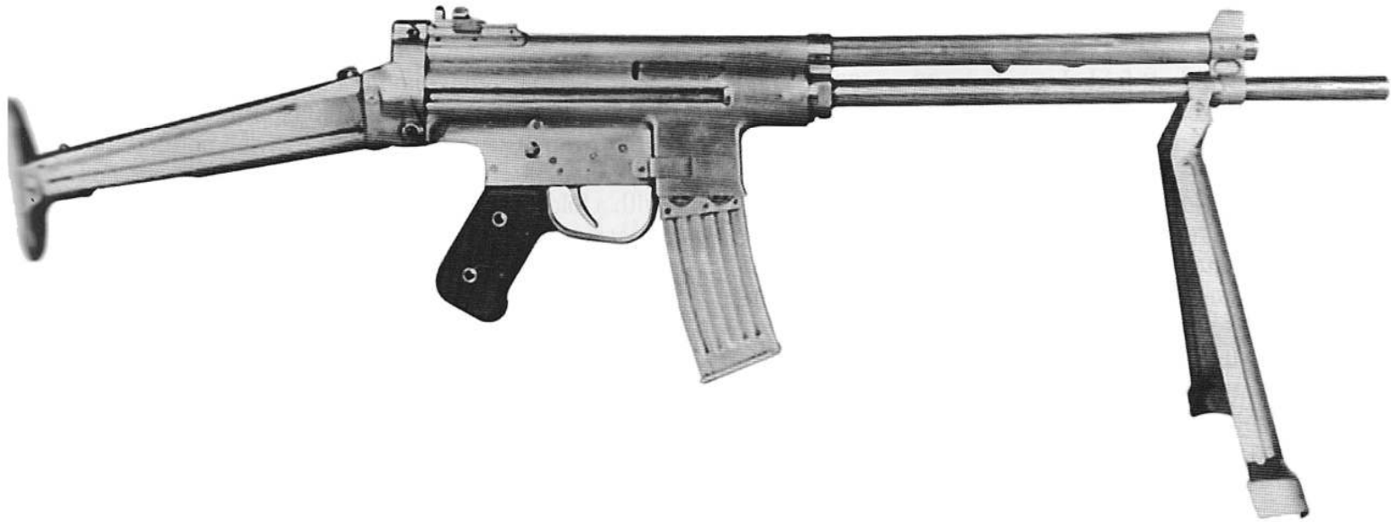
128. Right side view of the Löffler Model II/1 built to plan SKL 03, with butt and bipod extended, shown fitted with the early 30-round 7.65x35mm magazine.
