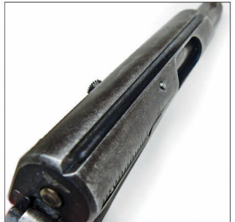
M1908 W&S auto with channel that acted as the rear sight.
