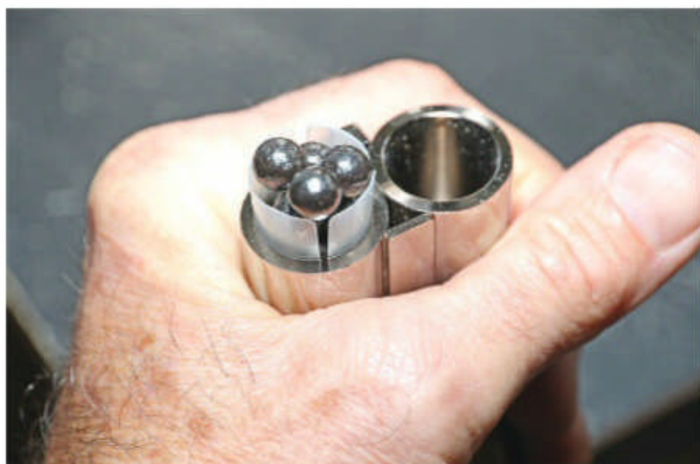
The wrong buckshot and wad combo gets you an irregular mess, and not a neat and orderly stacking.
