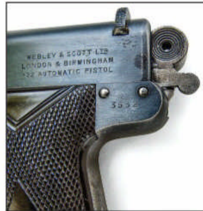
Close-up of the M1906 W&S hammer safety.
