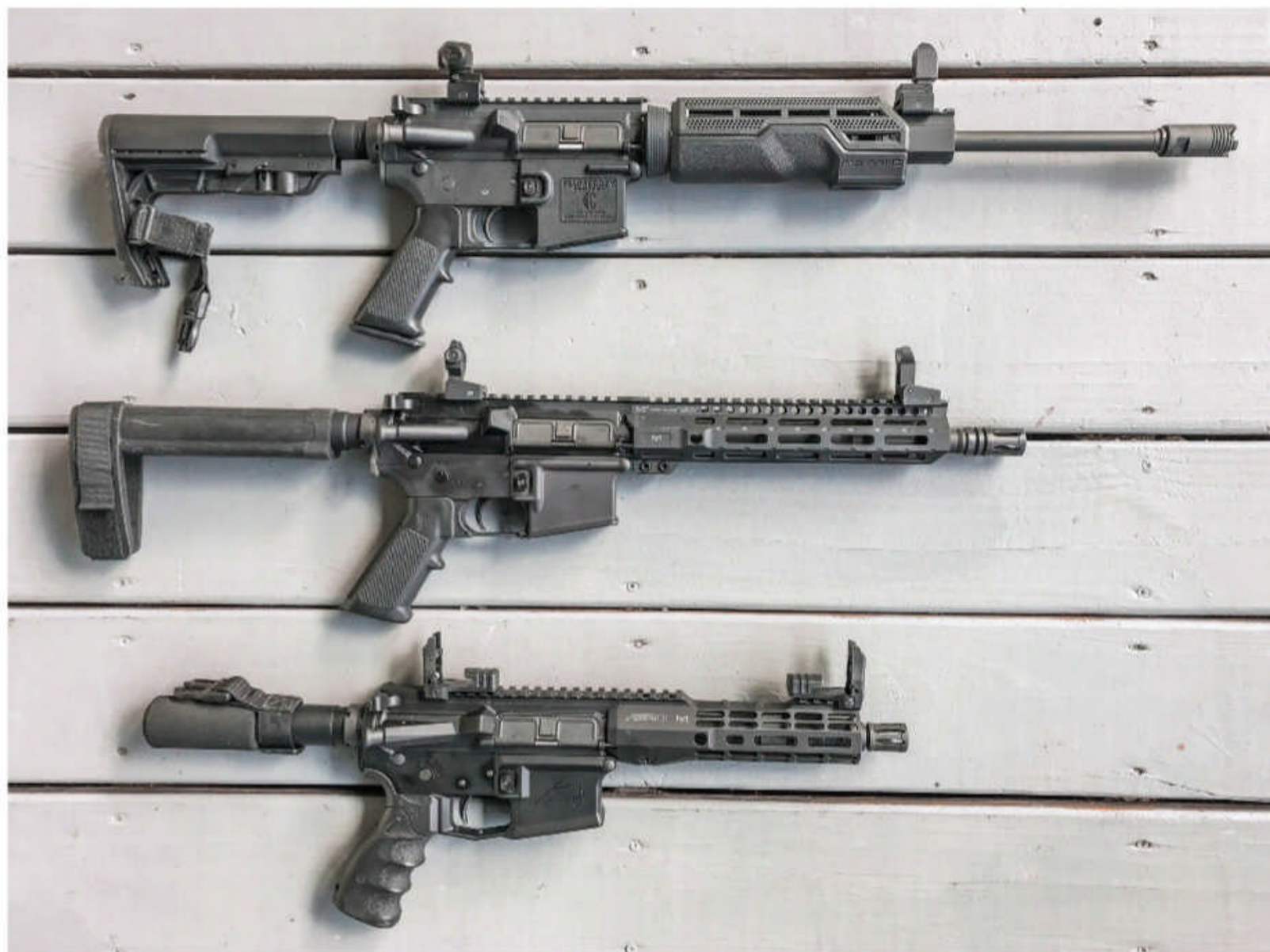
For comparison of length, here are three AR-15-type firearms: a lightweight AR-15 carbine with 16-inch barrel (TOP), 10.5-inch barreled AR-15 pistol (MIDDLE), and the Aero Precision M4E1 Atlas S-One with 7.5-inch barrel (BOTTOM).
