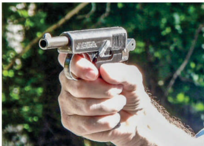
Firing the M1908 W&S .32 auto; note the safety is in the up position, which is "fire."
