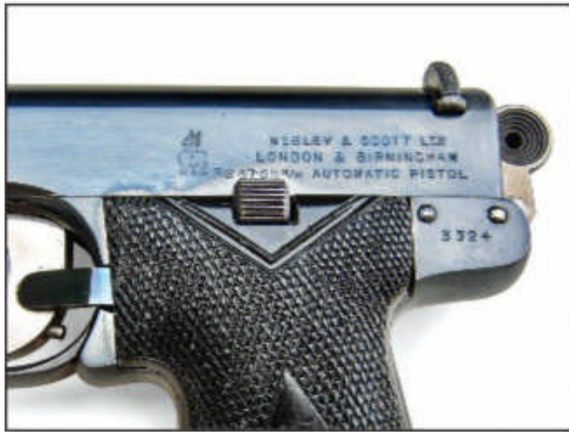
Close-up of the button safety on a M1906 W&S .32 auto.
