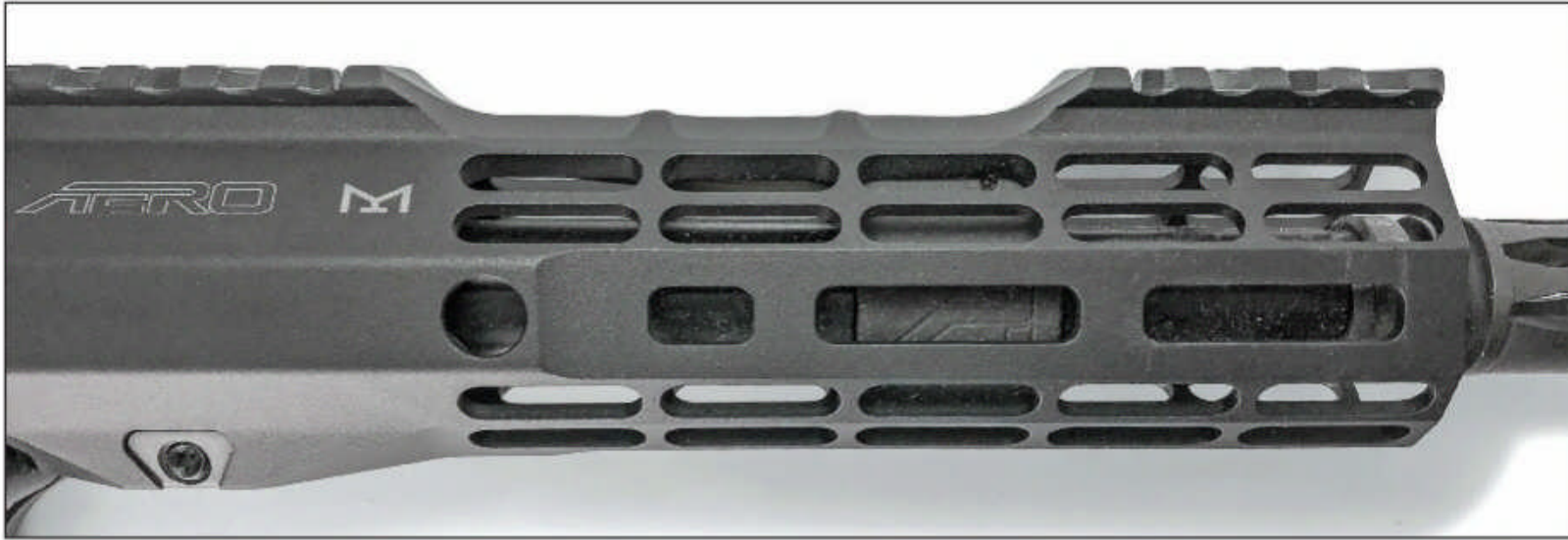
The free-float barrel shroud incorporates front and rear top Picatinny rails, multiple M-LOK positions, quick-disconnect sling sockets, and weighs only 4.9 ounces with only a 1.5-inch outside diameter.
