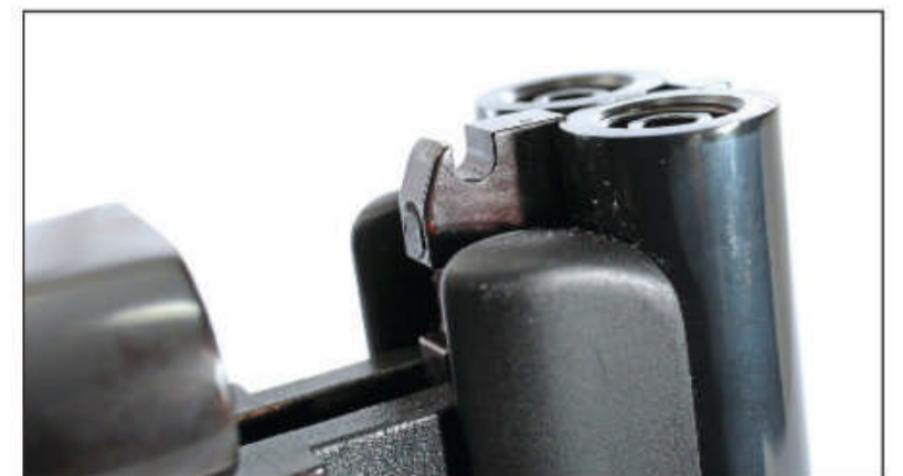
You can see the locking lug and its retaining notch, just below the chamber plugs, ready to receive a primer.
