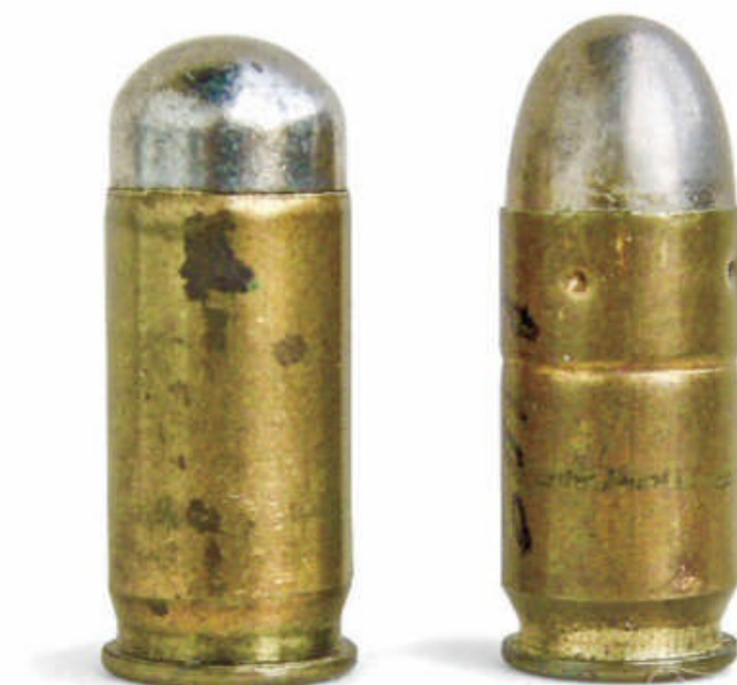
The .455 Webley auto cartridge at left compared to a .45 ACP cartridge at right.
