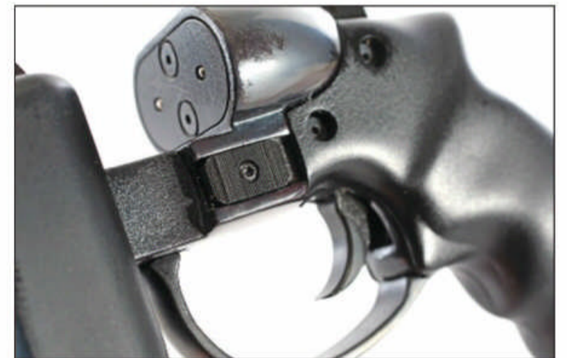
You can see the firing pins on the breechface, and the dual barrel unlocking tabs, the one above the trigger is the one on the left-hand side.
