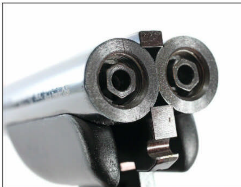
The charges are touched off by means of standard shotgun 209 primers, pressed into the rear of the chamber plugs.
