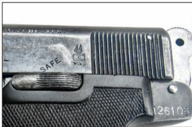
A W&S .32 auto with the lever safety that would become standard for the M1908 .32 auto.
