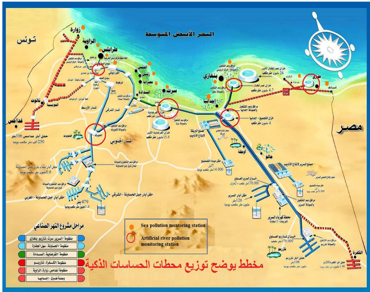
Figure 7. Smart sensors distribution for pollution monitoring on coast, and main tanks of artificial river
