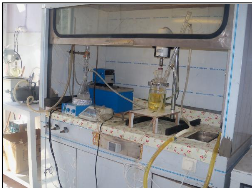
Figure 1. Experimental setup for biodiesel production
