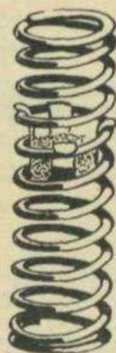
CANTRELL LUBRICATOR IN POSITION.
