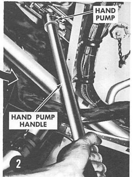
CONNECT HAND PUMP HANDLE TO HAND PUMP. (45 CYCLES TO FULLY OPEN CANOPY)
