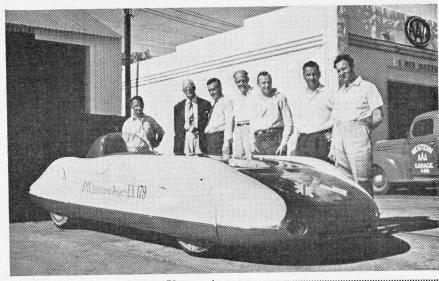
MINOR Streamliner: The EX179 record car which has just completed its successful attack on Class G speed records at Utah, powered by a 948 c.c. Series A B.M.C. engine. Capt. Eyston stands second from the left.
