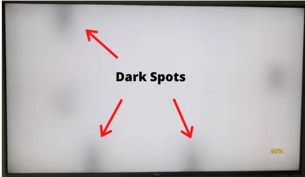
Fig 74. Heat Damage on LCD Displays
