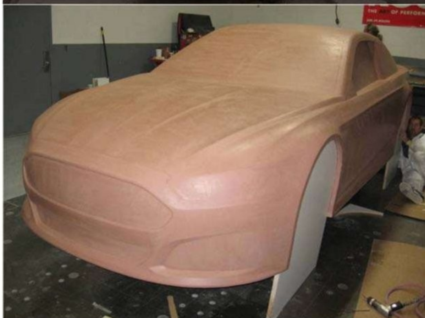
Ford used its time honoured clay modelling technique to develop the shape of its 2013 car. Though the greenhouse dimensions and certain other areas are specified by NASCAR and common to all cars, the rest was free
