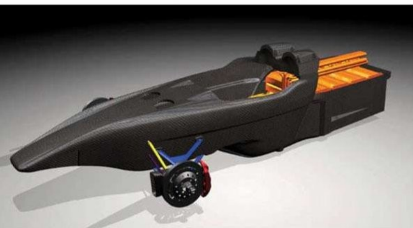
Unusually, the chassis uses two separate carbon monocoques, a standard tub built by Welter Racing and a second for the fuel cell
