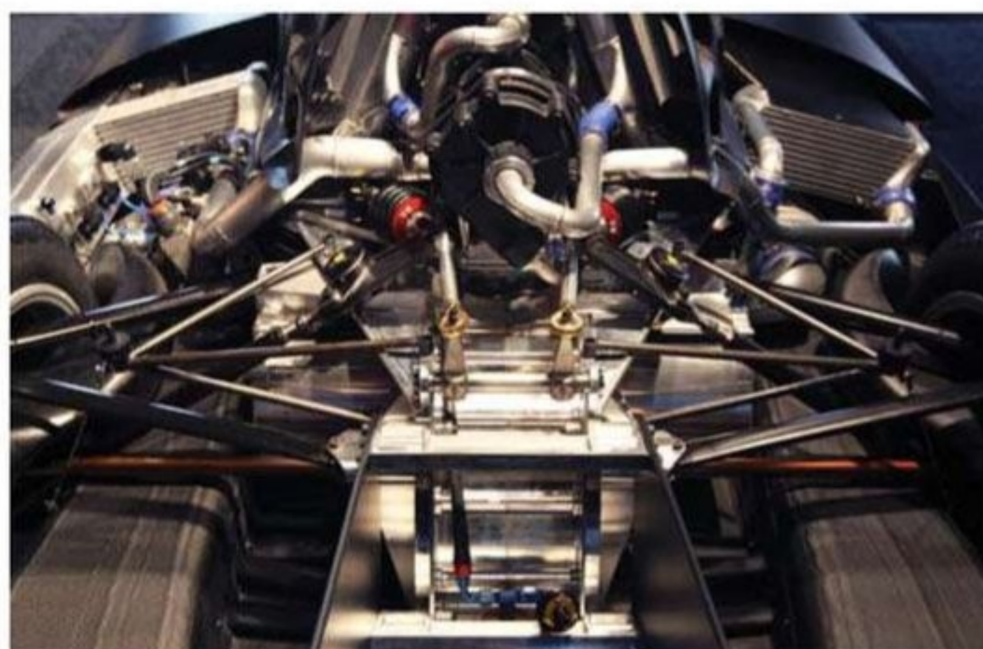
Rear suspension is conventional, but that's where it stops. Twin electric motors drive the rear wheels through a bespoke gearbox
