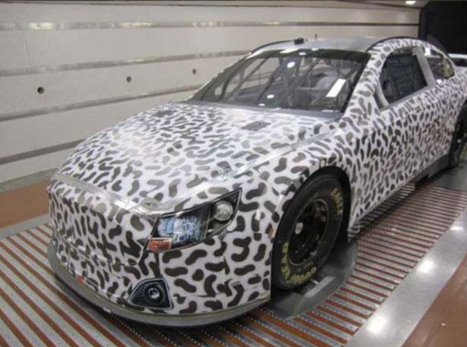
With the styling signed off, it was down to the aerodynamicists to develop the shape into a workable racecar. Wind tunnel facilities such as Aerodyn were used to develop the cars such as the Ford (above)
