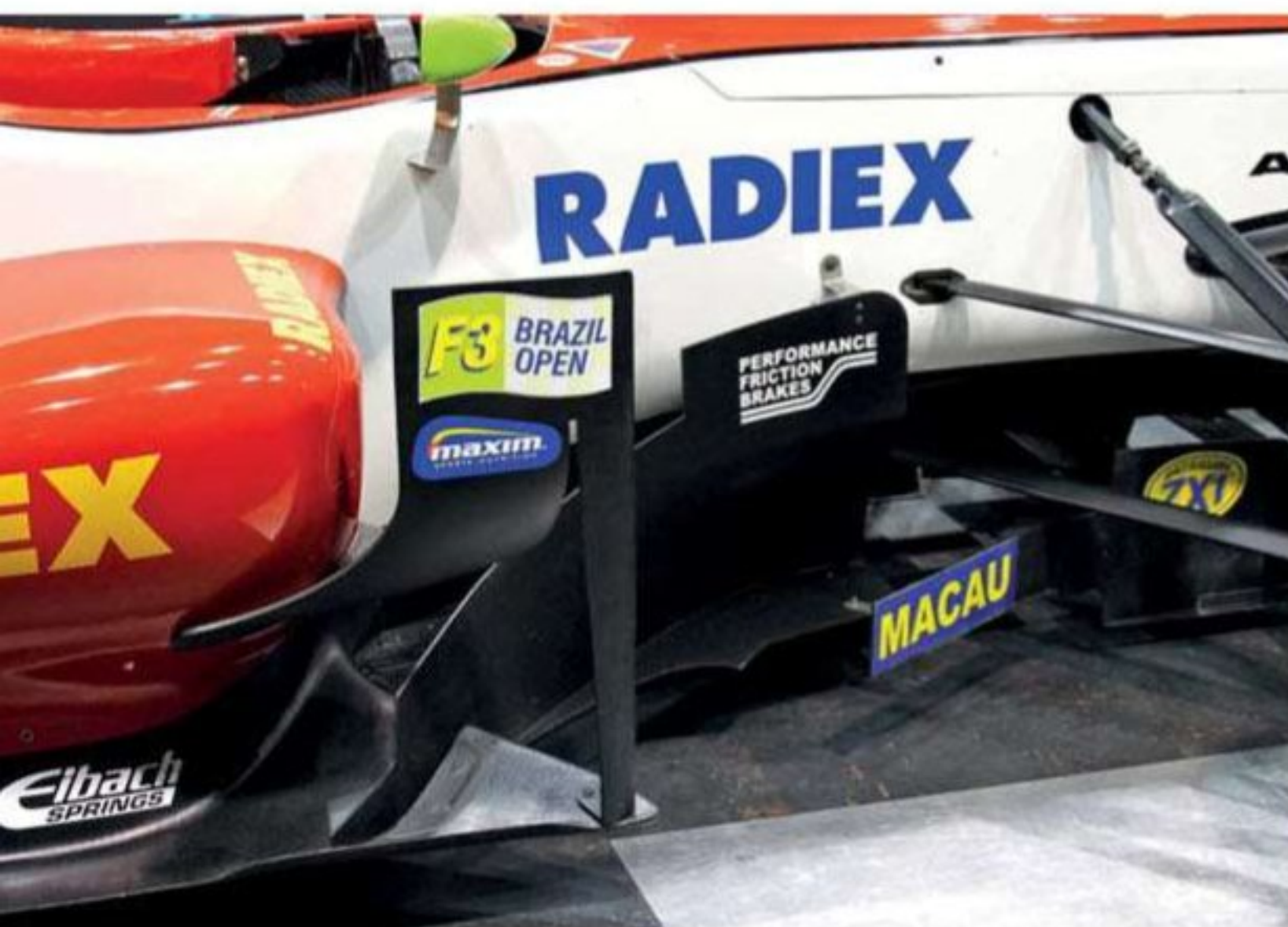
The F308 featured a medium height nose and lots of vortex-generating componentry under the nose
