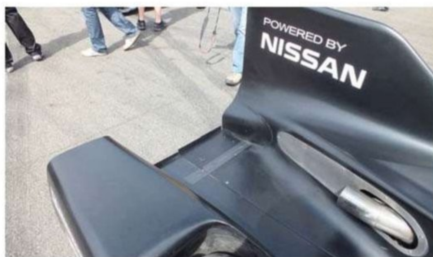
To alleviate the ACO's concerns about the car taking off in a spin, magnetic flaps were added at the rear, which deploy if the car goes backwards
