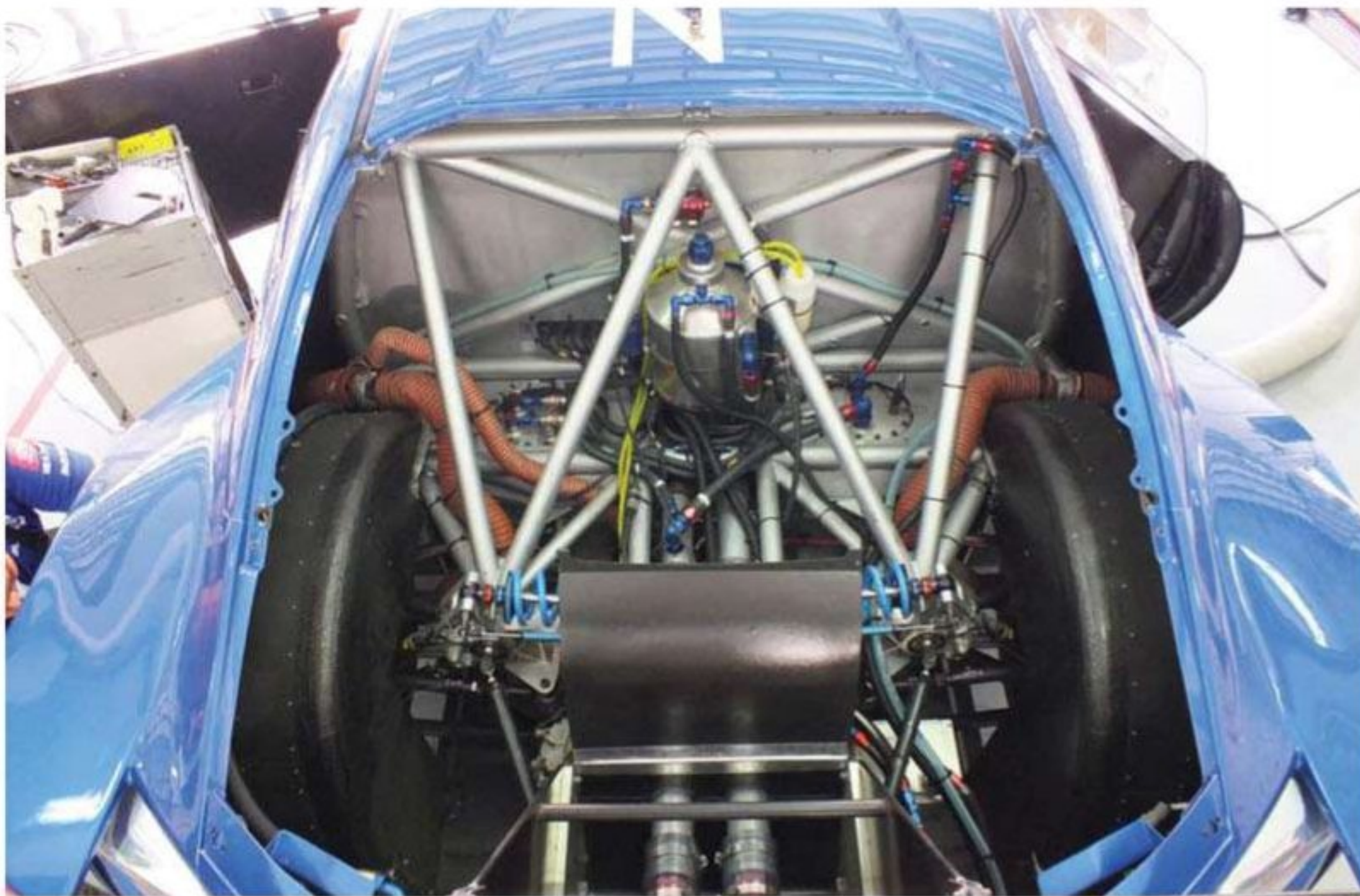
Rear suspension is traditional, with unequal length double wishbones and horizontally-mounted inboard dampers
