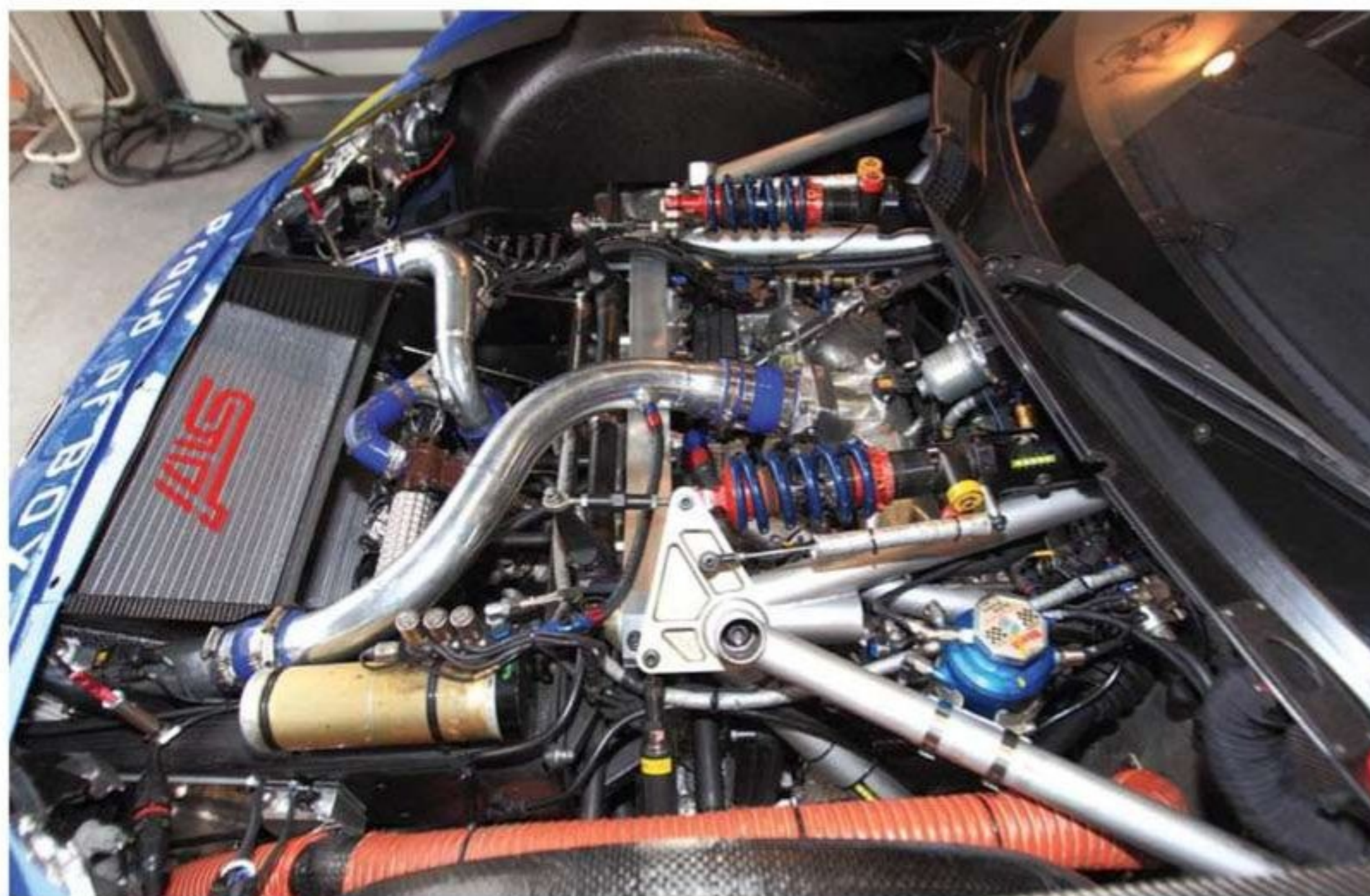
2.0-litre, turbocharged, EJ20 boxer engine is producing upwards of 350bhp. Dampers sit right above the engine
