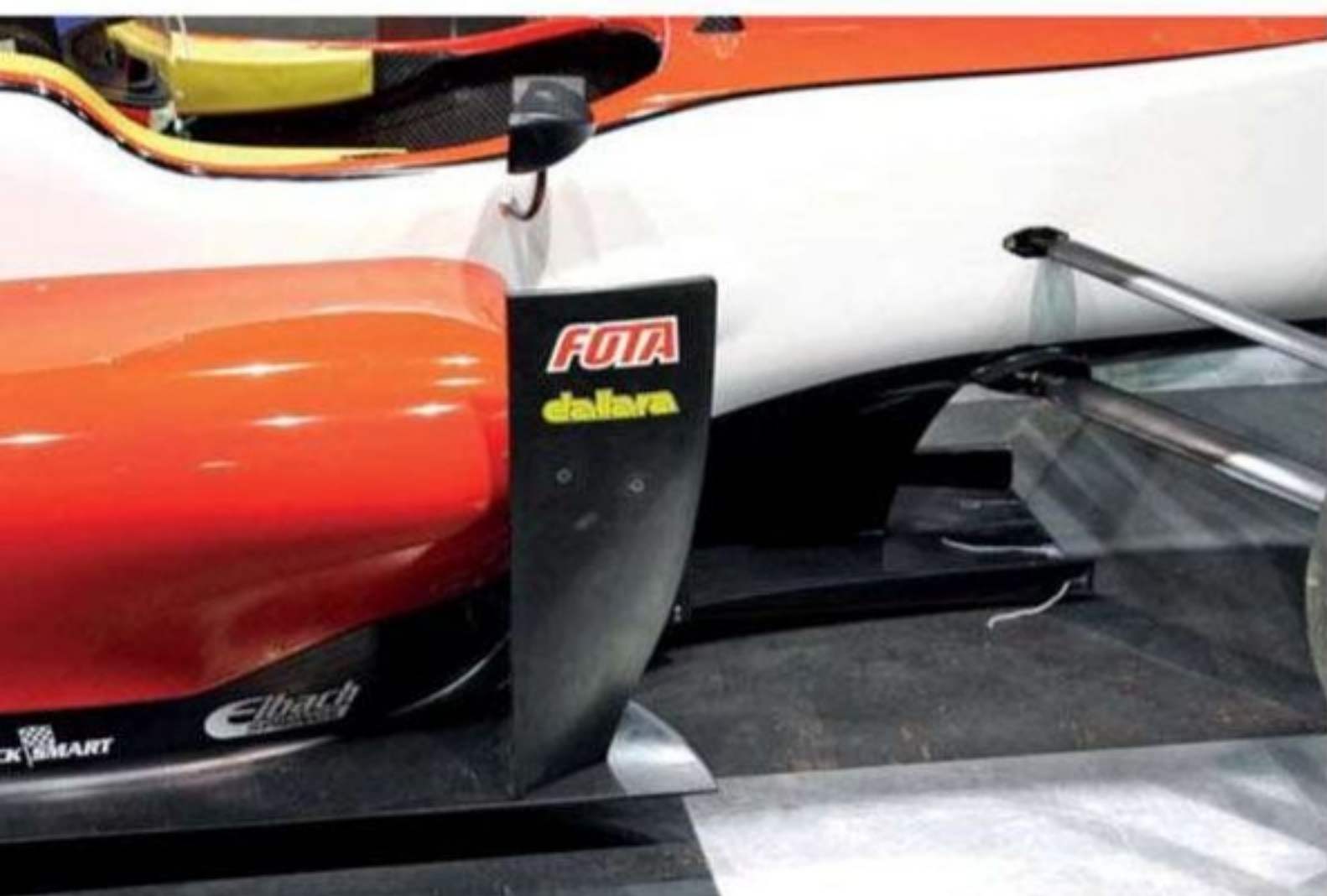
The new F3 regulations prohibit the use of aerodynamic devices in various regions around the car, so the F312's nose is higher but 'cleaner' beneath
