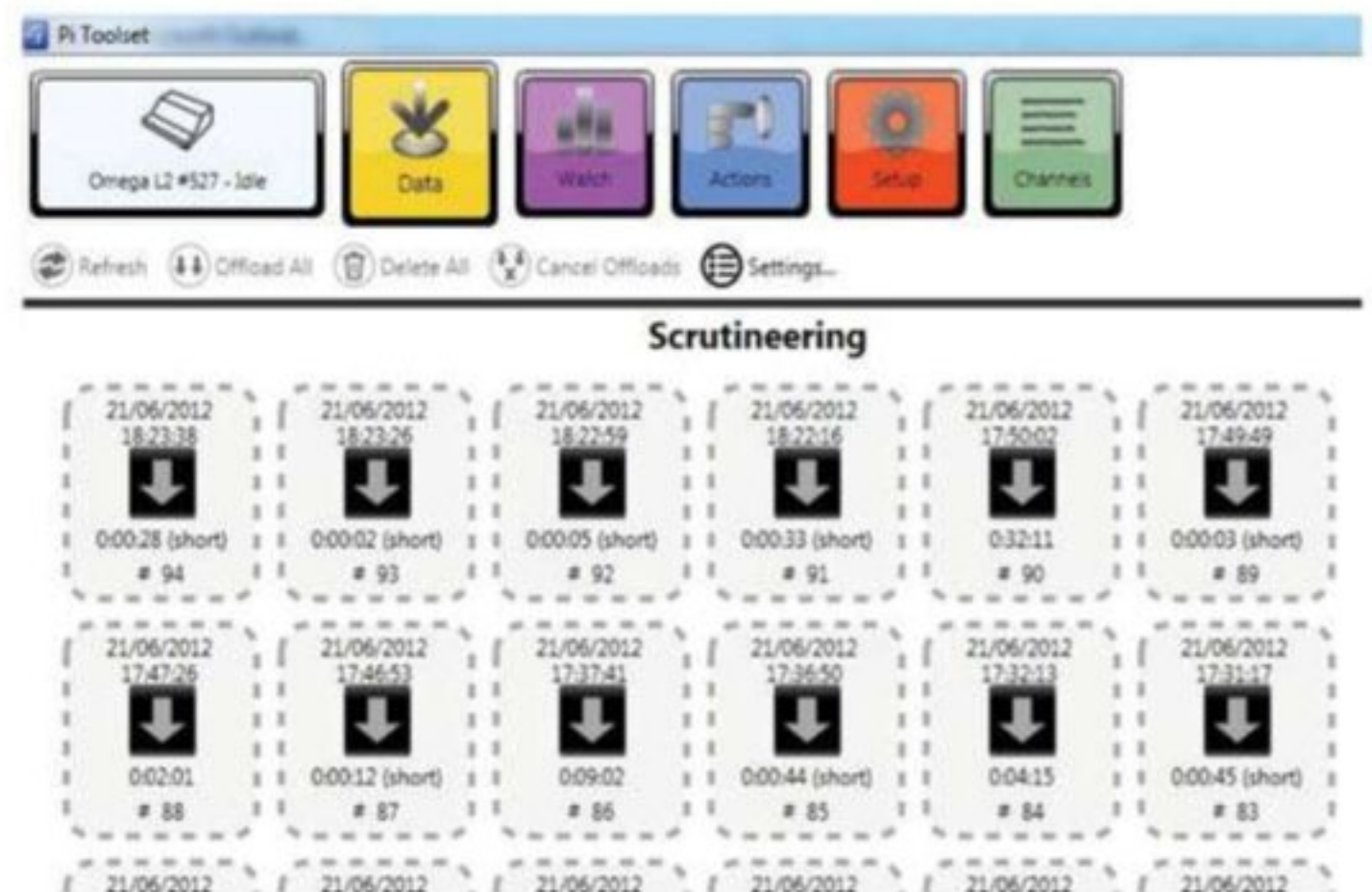
Figure 2: the scrutineering data can only be accessed by the scrutineer and, more importantly, can only be erased by the scrutineer
