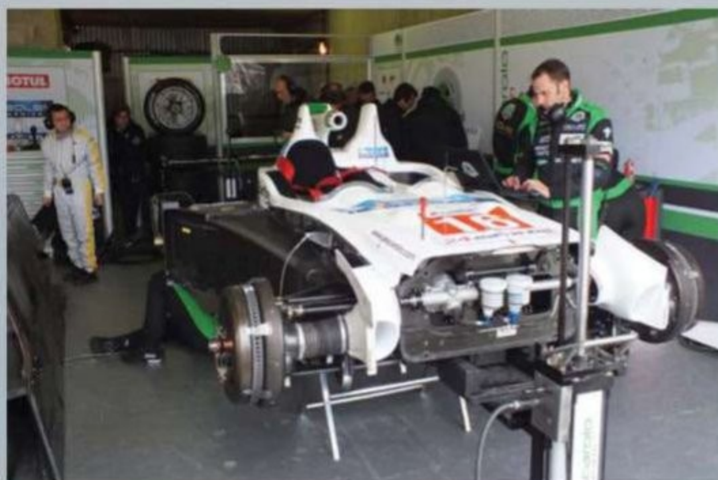
Though the chassis, suspension and gearbox all came straight from Aston Martin, the aerodynamics and cooling systems were all designed from scratch, including modifying the front suspension to suit the aero package
