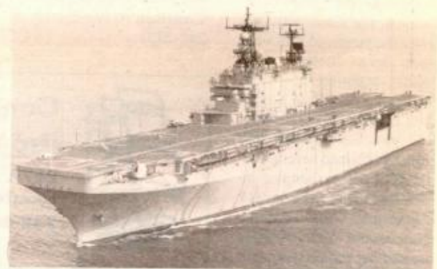
THE USS NASSAU (LHA-4) is an amphibious assault ship commissioned on July 28, 1979. The ship is 820 feet long and displacing 40,000 tons fully loaded, is capable of landing a fully equipped Marine Corps assault team by helicopter or landing craft, or a combination of the two.
