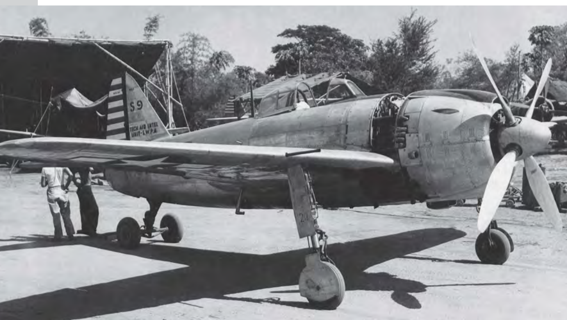
Coded S9, this aircraft was the second Shiden to be flown by the TAIU-SWPA, completing a number of sorties. USAAF and US Navy test pilots found the N1K1-J to be an excellent high-performance fighter, although its fragile landing gear was a major weakness. NATIONAL ARCHIVES AND RECORDS ADMINISTRATION
