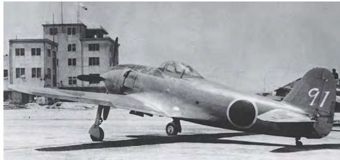
The prototype N1K2-J completed its first flight from the newly constructed Naruo airfield on 31 December 1943, with Kawanishi test pilot Munekichi Okayasu at the controls. Production aircraft differed very little from this machine, only the cowling and exhaust stubs being altered. The first 100 N1K2-Js also had the larger tail, as here. VIA PHILIP JARRETT
