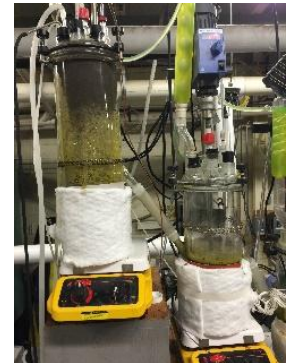
Continuous HCl Leach Pilot
