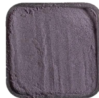
Met-spar grade concentrate (~69% CaF 2 ) produced from Ashram Deposit
