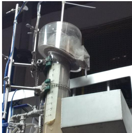
3 inch column flotation Pilot
