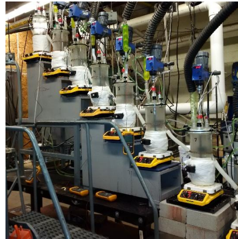
Continuous HCl Leach Pilot
