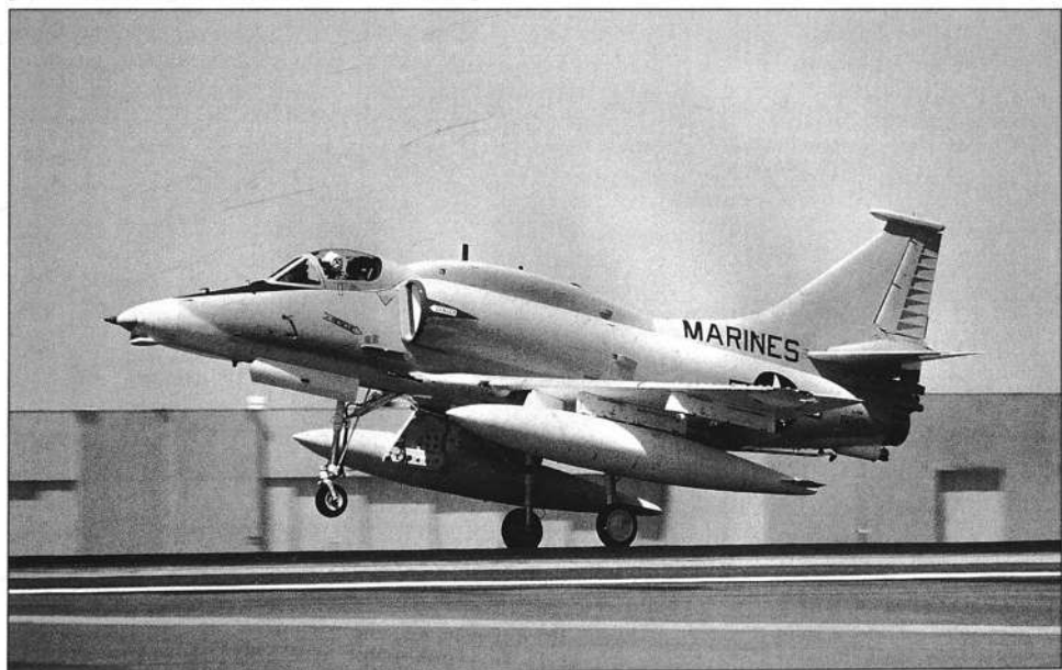
A-4M Bu.No.159471 of the USMC showing the distinctive humped avionics compartment first retrofitted to A-4E Skyraiders. The A-4M was the last version used by the US. Total A-4 production reaching 2,960, including overseas deliveries of new and surplus Skyhawks to the air forces of Argentina (A-4P), Singapore (A-4S), Israel (A-4H/N), Kuwait (A-4KU), Malaysia (A-4PTM), Australia (A-4G) and New Zealand.
