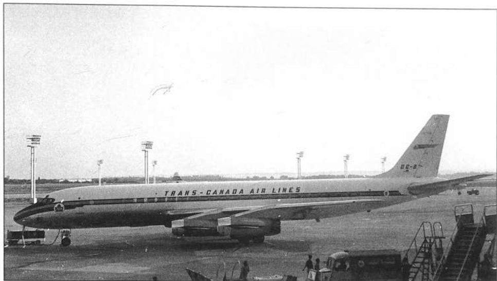
DC-8-41 CF-TJA of Trans-Canada Airlines. A total of thirty-two Series 40s, all powered by Rolls-Royce Conway turbo fans, were built for Alitalia, Canadian Pacific and Trans-Canada.
