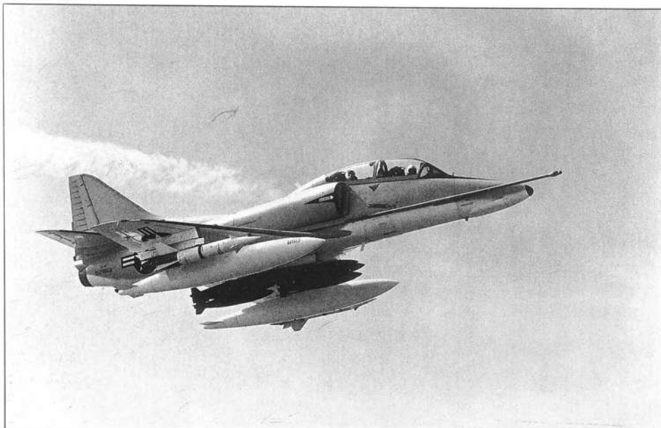
TA-4F Bu.No.152850, showing the distinctive starboard-mounted air-refuelling probe. The majority of TA-4Fs built were later modified as TA-4Js, others becoming EA-4F 'electronic aggressors' and OA-4M tactical air co-ordinators for the USMC.
