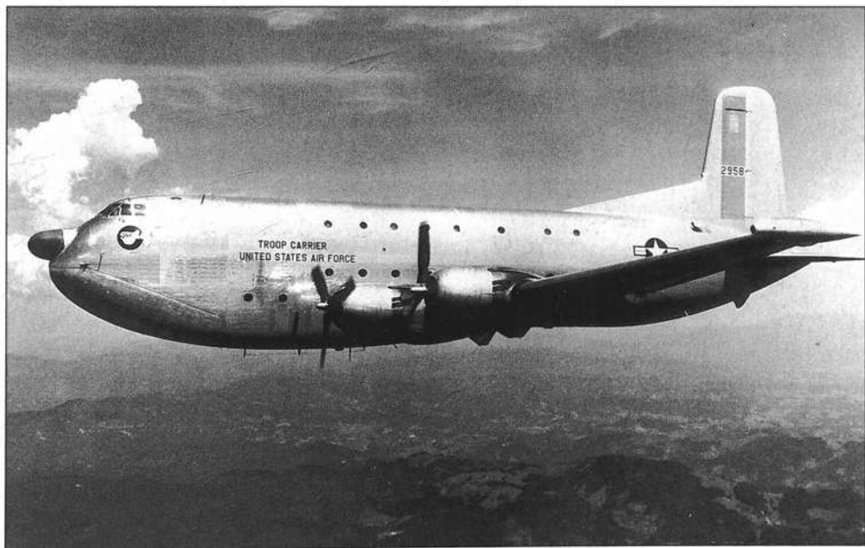
C-124C 52-958. The C-124C differed externally from the C-124A in having 3,800hp Pratt & Whitney R-1460-63A engines and the APS-42 Weather Search Radar in a nose radome. Some 243 C models were produced at Long Beach, taking the final total of Globemaster IIs built to 448.
