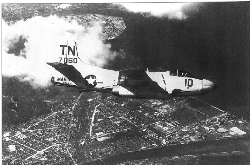
Some 261 F3D aircraft were built and they served from 1950 until the Vietnam War. Pictured is F3D-2Q (EF-10B) Bu.No.127060 of VMCJ-3, USMC, one of thirty-five F3D-2s modified as ECM aircraft.
