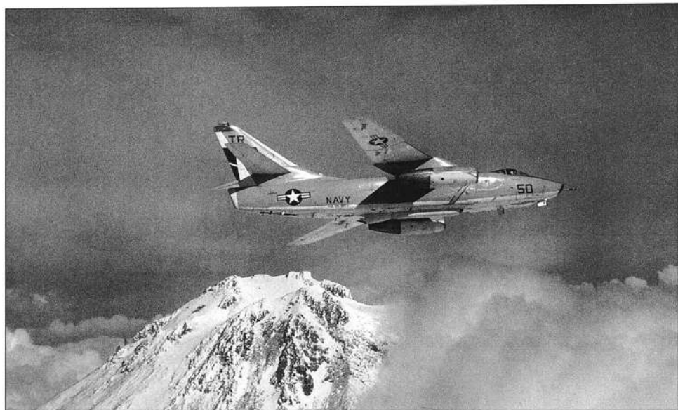
Bu.No.142650 of VAQ-135 Det 1, one of thirty-nine EKA-3B combination ECM/tanker aircraft (thirty-four of which were modified from KA-3B tanker configuration by the Naval Air Rework Facility (NARF) at Alameda, in northern California). After 1975 most EKA-3Bs had their electronic equipment removed and were re-designated KA-3Bs.
