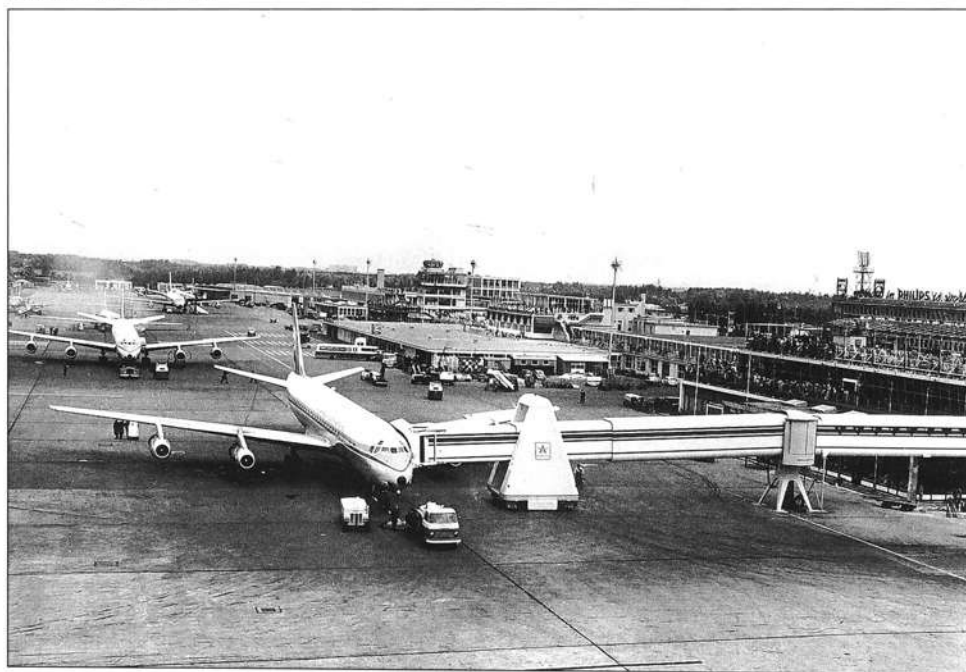
DC-8-30s and -50s of KLM at Schiphol. The DC-8 Series 50, which first flew on 20 December 1960, was the first DC-8 to be powered by turbo fan engines instead of turbo jets, and entered service with KLM on 3 April 1961.
