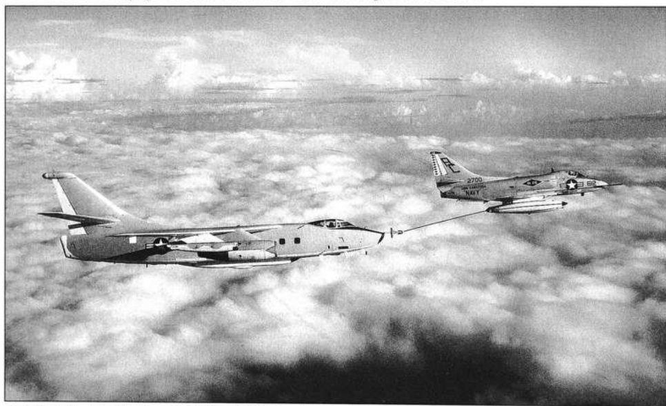
A-4D-2 (A-4B) Skyhawk Bu.No.142700 of VA-216 refuels an EA-3B (A3D-2Q) Skywarrior of VQ-2 over the Mediterranean on 26 October 1967. Both squadrons were part of CVW-3 stationed aboard the attack aircraft carrier USS Saratoga (CVA-60) during her 1967 Mediterranean deployment. Some twenty-five A3D-2Q/RA-3B versions were built and they could be easily distinguished externally by the ventral 'canoe' fairing and square windows on the fuselage sides.
