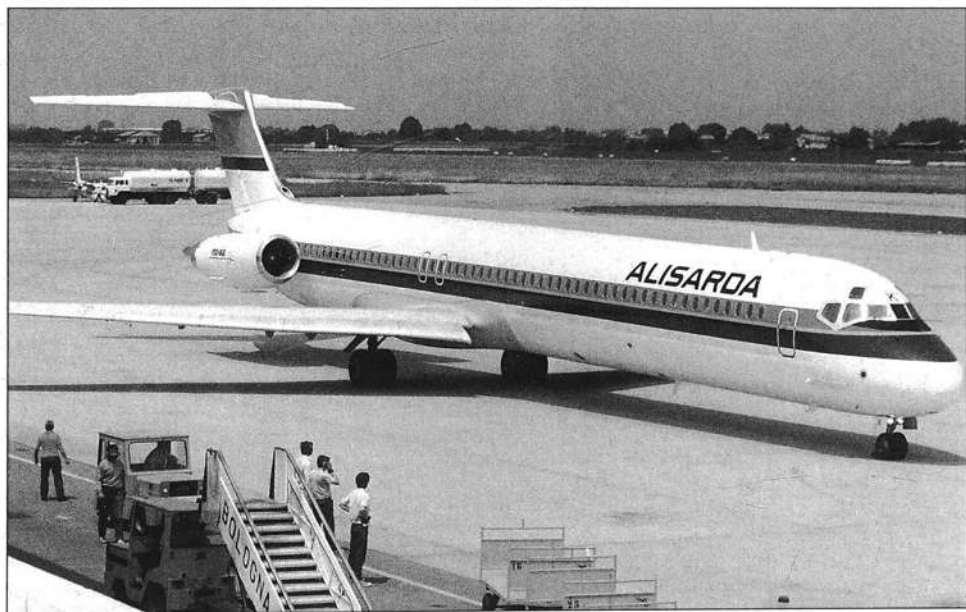
The first Series 80 (or Super 80), a stretched version of the DC-9 with re-fanned engines and updated avionics, was the 909th DC-9 off the production line and was first flown on 18 October 1979. At first, sales of the DC-9-80 were slow, but attractive short-term lease deals led to an upsurge in interest. The DC-9-82 (MD-82) was first flown on 8 January 1981. Starting in 1983, McDonnell Douglas began officially referring to the DC-9-80 as the MD-80. Pictured is MD-82 HB-IKK (now I-SMEL) of Alisardia (now Meridiana) at Bologna on 30 May 1985.
