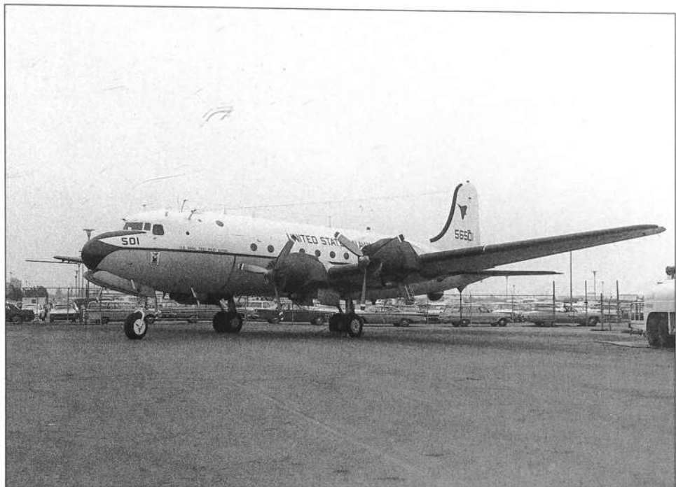
R5D-3 (C-54Q) Bu.No.56501, one of eighty-six C-54Ds transferred from the USAF to the USN. Most surviving R5D-3s were re-designated C-54Qs in 1962.
