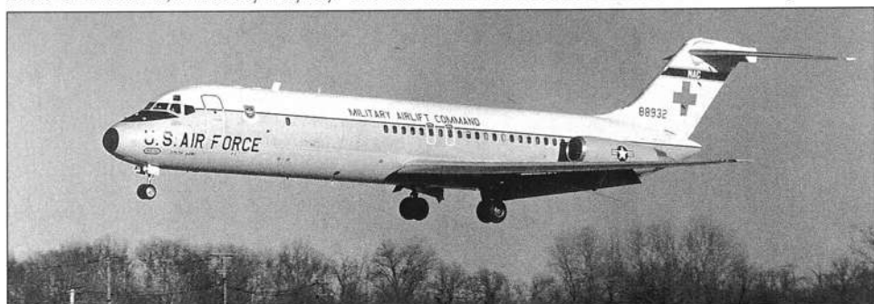
All three services of the US military operate the DC-9. In USAF service, twenty-three C-9A Nightingale aero-medical evacuation aircraft (derivative of the DC-9 Series 20 airliner) can each carry forty patients plus five medical staff. Pictured is C-9A 68-8932 of the 375th Aeromedical Airlift Wing of MAC in the US.
