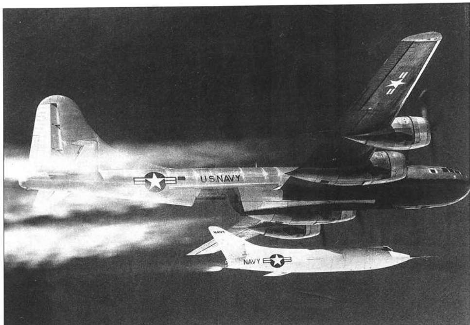
The D-558-II Skyrocket research aircraft, one of three built and the first aircraft to exceed Mach 2, air-launched from P2B-1S (B-29) on 4 February 1951.
