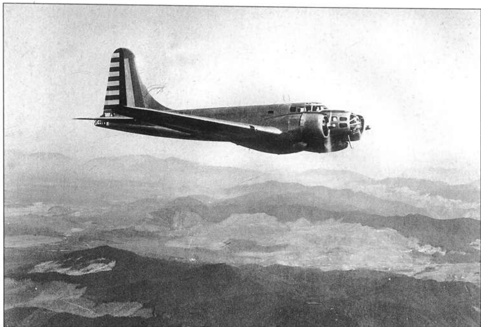
The B-23 Dragon, pictured here on 29 August 1940 over Mt Rainier, was an improved B-18 with a redesigned fuselage and, for the first time in an American bomber, a tail-gun position. Thirty-eight B-23s were ordered and the first flew on 27 July 1939. Most were used for a brief interlude on Pacific coastal patrol before being relegated to training and transport roles.
