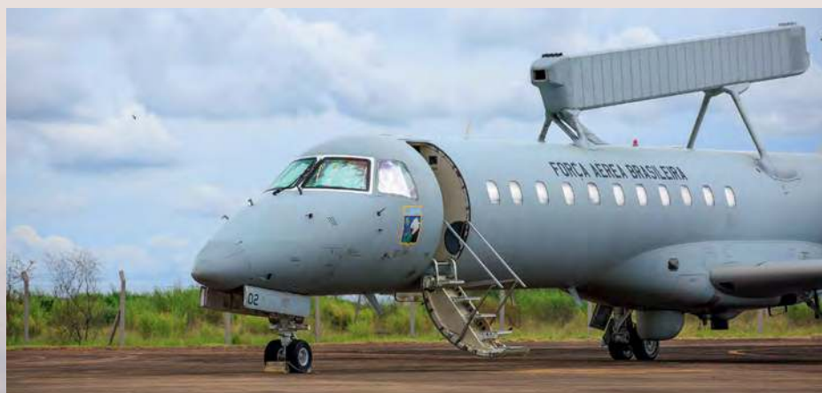
Above: The E-99 AEW&C aircraft is a vital part of the operation. This example wears the insignia of 2 o /6 o GAv 'Guardião'. The Anápolis-based unit flies five such aircraft. André Feitosa and Johnson Barros/Brazilian Air Force
