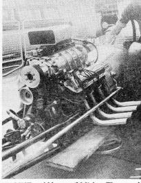
ENGINE and blower of Mickey Thompson's Dragster. It is a Ford Galaxie unit restroked and bored to 8,000 c.c., and uses methanol fuel.
