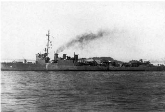
Left: USS Zane (DMS 14), which ran aground at Honiavasa Passage in the early morning of June 30, was commissioned in 1921 as a Clemson-class destroyer. She was converted to a high-speed minesweeper in 1940 and was a veteran of Pearl Harbor and Guadalcanal. Following the grounding at Honiavasa, she was repaired at Mare Island and served in the later campaigns in the Marshalls and Marianas. (Photo supplied via Joseph E. Gunterman, a member of the Zane's crew in WWII.)
