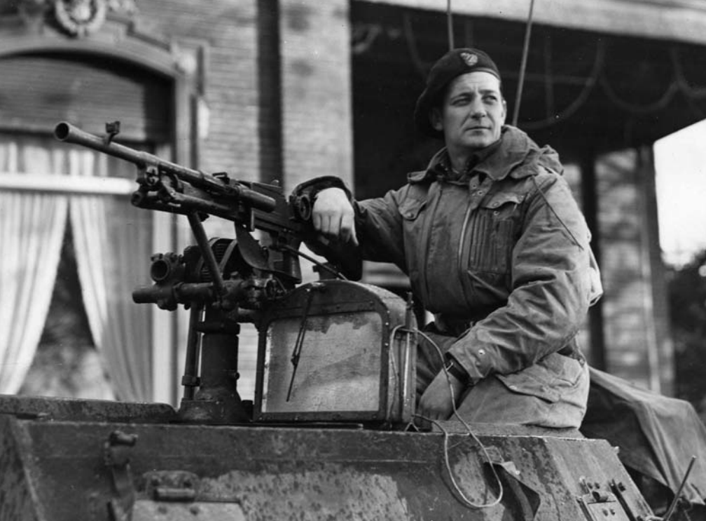
A Canadian officer is shown with a Bren gun in a Humber Mk. I armored car. The Bren gun, the principle machine gun of British/Commonwealth infantry, fired .303-inch ammunition.
