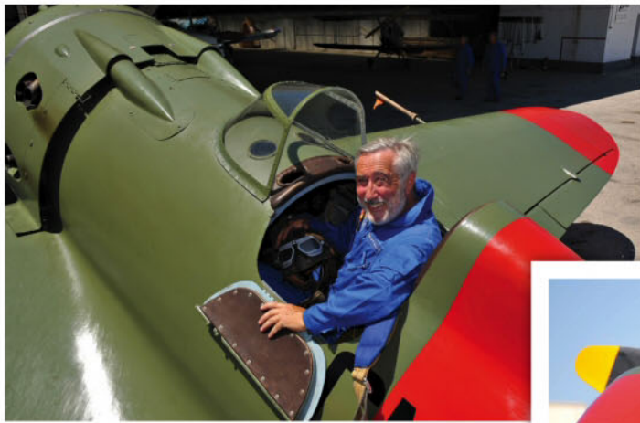
The aircraft replicates an I-16 Type 10. The Type 10 was powered by a Shvetsov M-25B, a licence-built Wright Cyclone.
