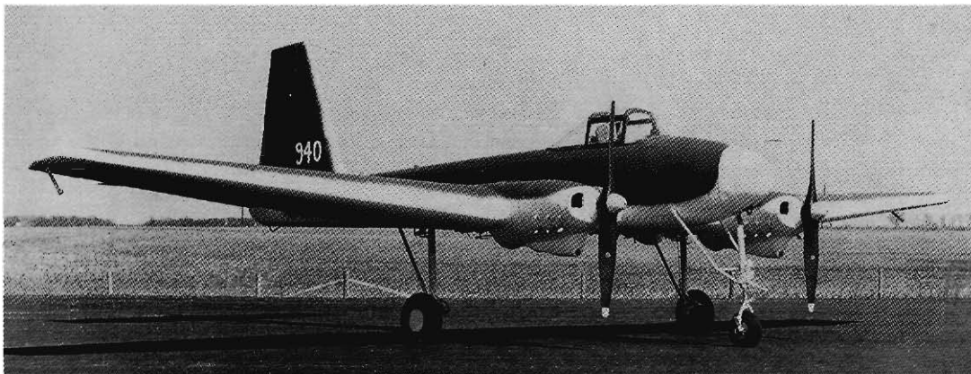
The Interstate TDR was nothing more than an oversized radio controlled model aircraft. (Credit: National Archives)
