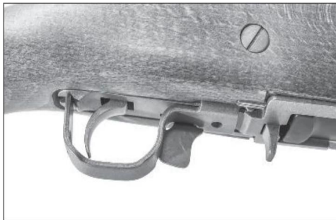
The safety is a blade forward of the trigger guard. Push it forward to make the Mini ready to fire.
