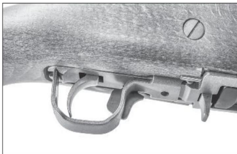
Pulled to the rear, the safety locks the trigger mechanism, and readily determined by touch.
