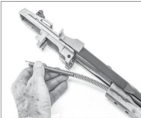
And then ease it relaxed and pull it out of the charging handle.
