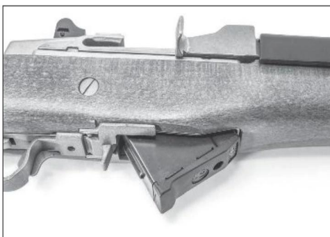
Locking a fresh magazine in place means hooking the front and then swinging the magazine up until it latches in place.
