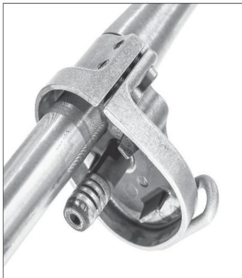
The "piston" is just a spigot, and blows the charging handle off of the gas system.
