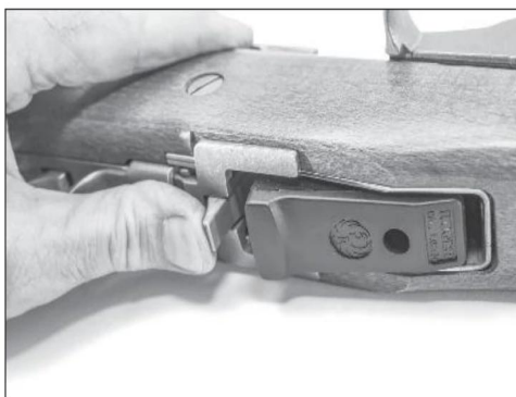
To remove the magazine, push the magazine catch lever forward.
