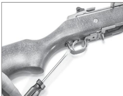
To disassemble, pivot the rear of the trigger guard down. Often, a screwdriver is a big help in mustering the necessary leverage.
