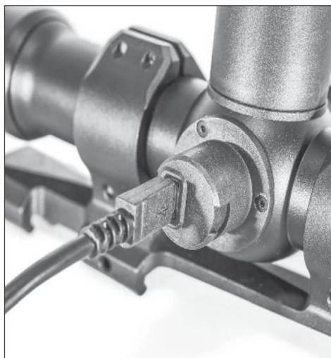
Here is the XM50 internal battery being charged.
