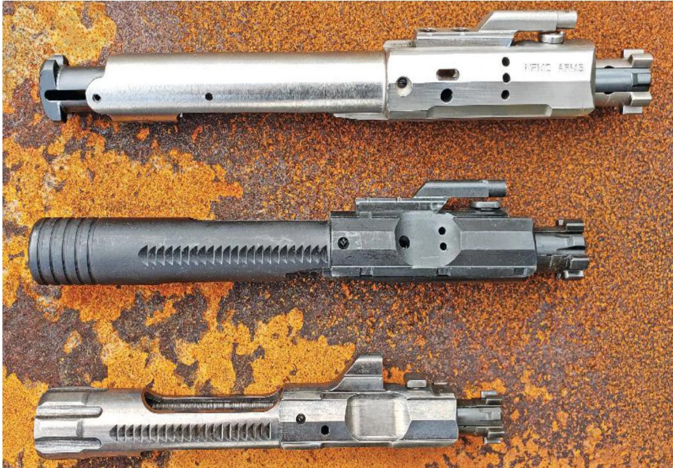
A look at the large NEMO Arms .300 Win. Mag. bolt and bolt carrier (TOP) with its built-in buffer system, compared to a S&W M&P 10 .308 bolt and bolt carrier (MIDDLE), and a 5.56 bolt and bolt carrier from LWRC (BOTTOM).
