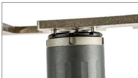
The SilencerCo tool, unscrewing the rear cap of the Omega 300.
