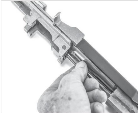
Pull the recoil spring assembly out of the retaining cup.
