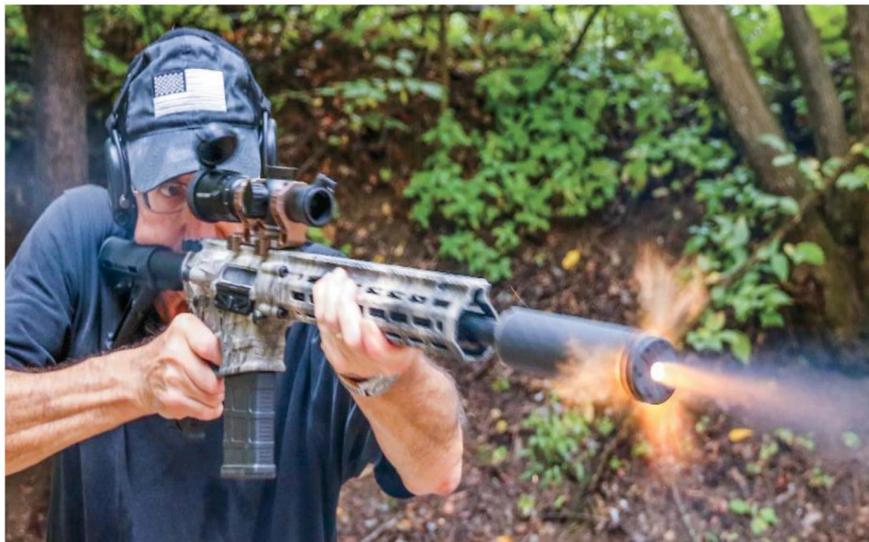
Suppressors tame the noise, but the gases that come out are still hot. And they can cause flash under the right circumstances. Here we see the Anchor Brake doing its job.
