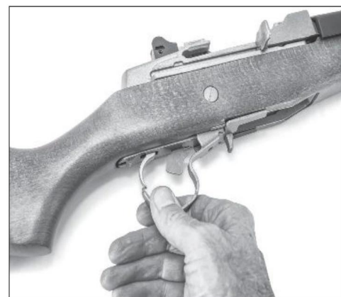
Pull the trigger assembly down out of the stock.
