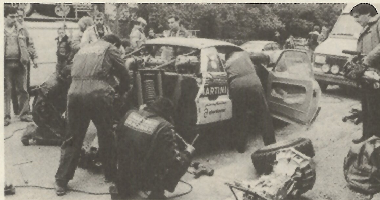
The Lancia mechanics change the gearbox on the Lancia Rally of Jean-Claude Andruet.
