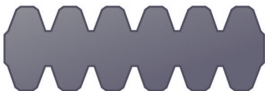
33 - Cross section of a double-sided poly-V-belt
