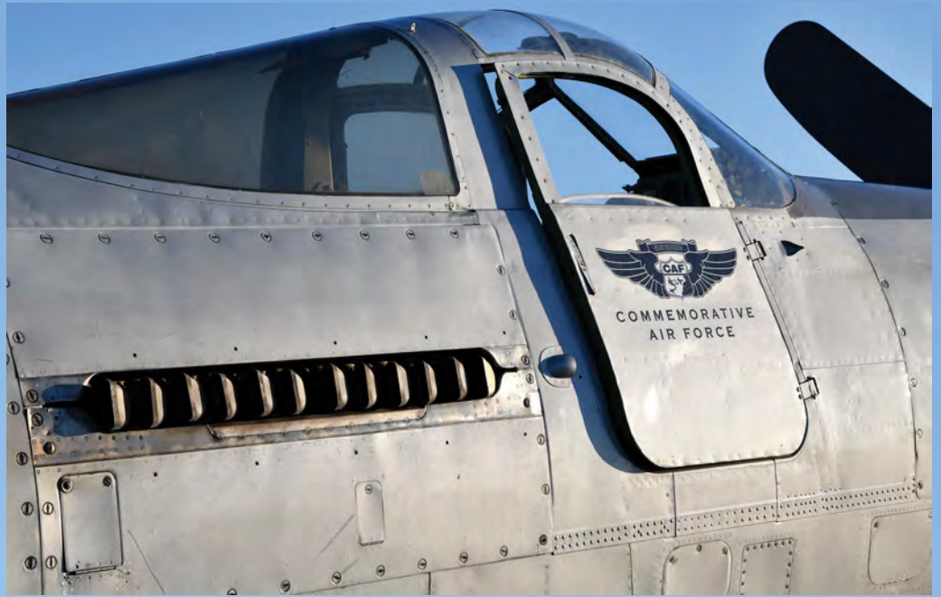
ABOVE: The Kingcobra shows off the somewhat unorthodox method of crew entry favoured by the Bell designers.
