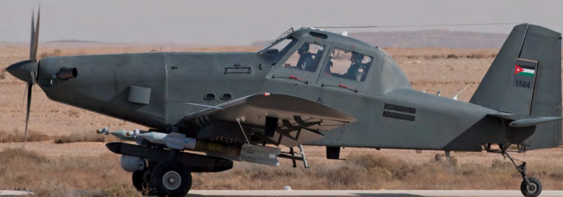
One of ten IOMAX Border Patrol Aircraft (not an Archangel) in service with the Royal Jordanian Air Force. This example, serial number 1584, is loaded with two GBU-12 laser-guided bombs and the IOMAX mission pod fitted with an MX-15Di imaging system. Arnold ten Pas
