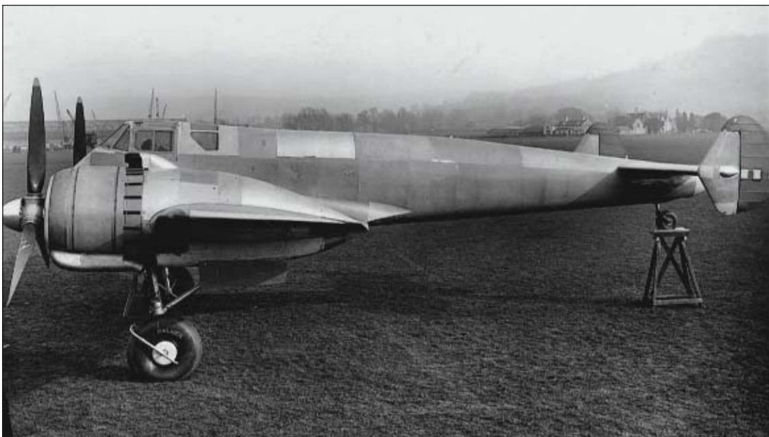
LEFT A side view of the newly-completed first prototype at Gloster's Brockworth airfield. Note the doped, fabric-covered rudders and the factory under construction in the background on the left. This is photo 10146D, taken in early April 1939.
