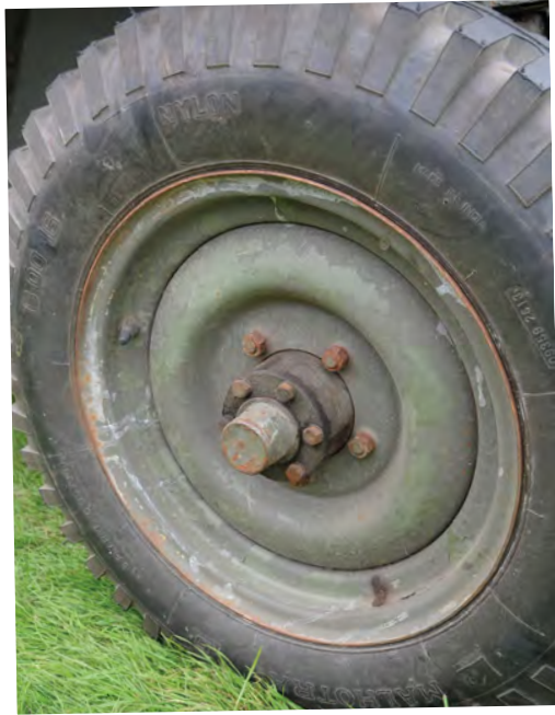
Above: The M201 was fitted with conventional well-base drop rims; the original radial tyres on this example have been replaced by 6.00-16 bar-grips. Right: Lightly-Americanised Hotchkiss M201 up for sale at the recent War & Peace Revival.
