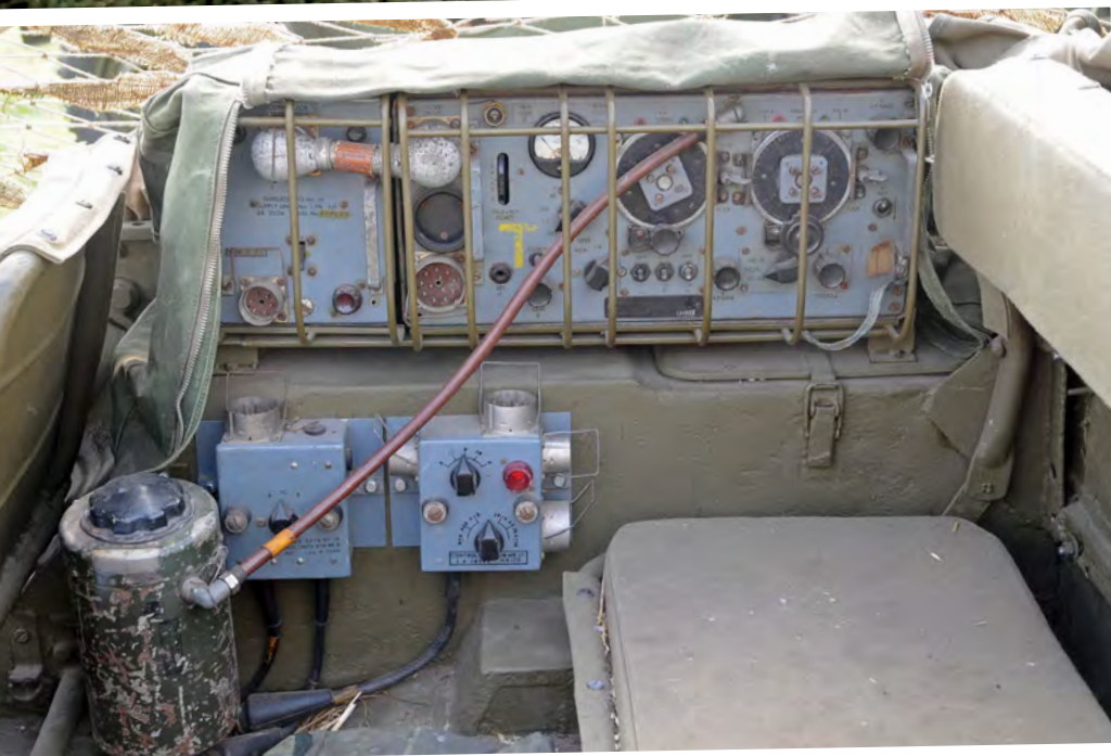
Above: British Number 19 wireless set fitted to the right-hand rear mudguard.
