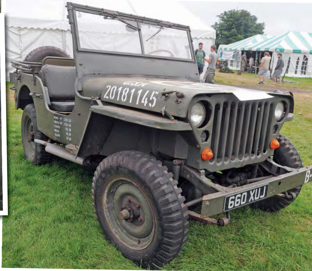
Above: The M201 was fitted with conventional well-base drop rims; the original radial tyres on this example have been replaced by 6.00-16 bar-grips. Right: Lightly-Americanised Hotchkiss M201 up for sale at the recent War & Peace Revival.
