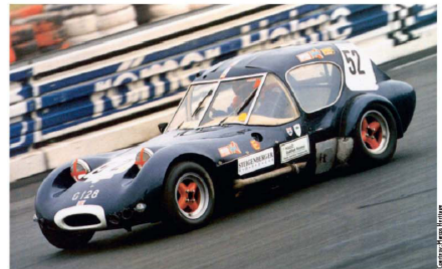
The gulfing Marcos sports coupé, otherwise known as the Ugly Duckling, successfully used a wooden chassis
