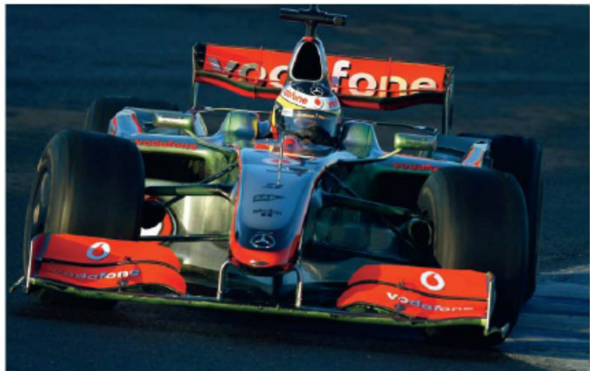
The final version of the MP4/23(K), also fitted with KERS. Note here the green dye coating for flow visualisation
