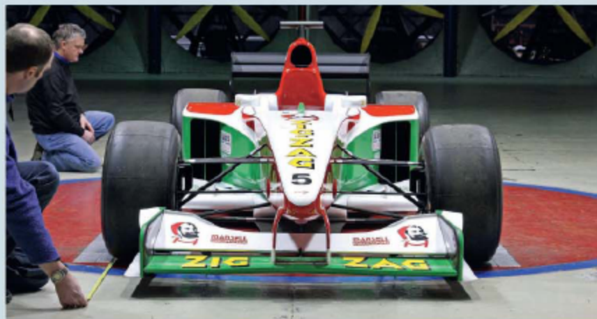
The Mansell Motor Sport EuroBOSS Benetton B199 being set up in the MIRA wind tunnel
