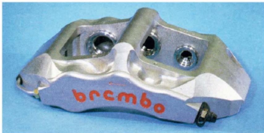
As well as pistons, AIBe also had nothing but positive benefits for use in brake calipers, which were found to be both lighter and stiffer, pleasing both drivers and engineers. Shown is a 1997 Formula 1 caliper from Brembo
