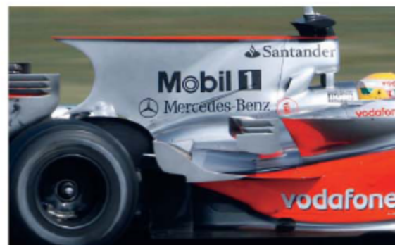
At the German Grand Prix, the MP4/23 was fitted with the so-called 'amwif' wing, designed to increase stability in a lateral wind
