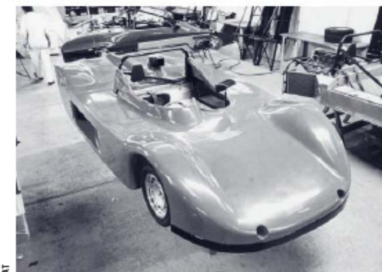
Ashmore's 1985 Sports 2000 racer, the T594, embodied his two design philosophies perfectly - a chassis as stiff as possible and a body as aerodynamic as possible. The teardrop-shaped car proved to be a success
