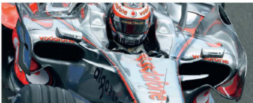
At Silverstone the cars ran with asymmetric radiator ducts. The team also introduced the small blades on the sides of the chassis ahead of the cockpit at the French Grand Prix (NB Ferrari and Renault also employed similar devices)
