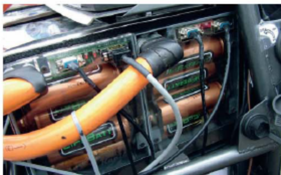
The all-electric UH12A has 240 LiFeBATT lithium-iron phosphate cells, which provided more than enough power to finish the Endurance section
